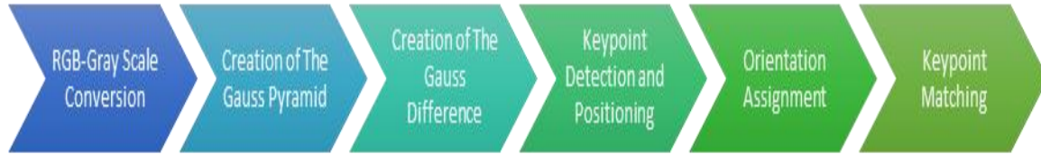
Figure 4.3. SIFT algorithm flowchart
