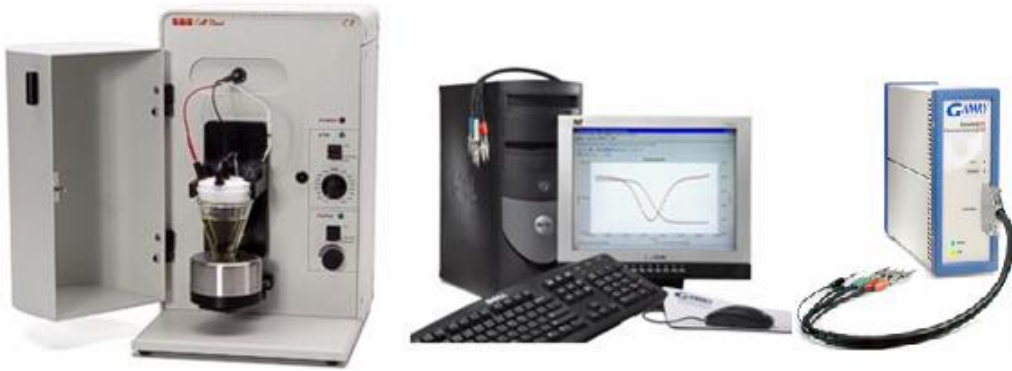
Şekil 3.1. Bioanalytical System C3 hücre; Gamry Referans 600 ve 750 potantiyostat/galvanostat/ZRA
