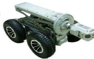
Figure 3.1. Camera and Robot used in photographing inside the pipe
