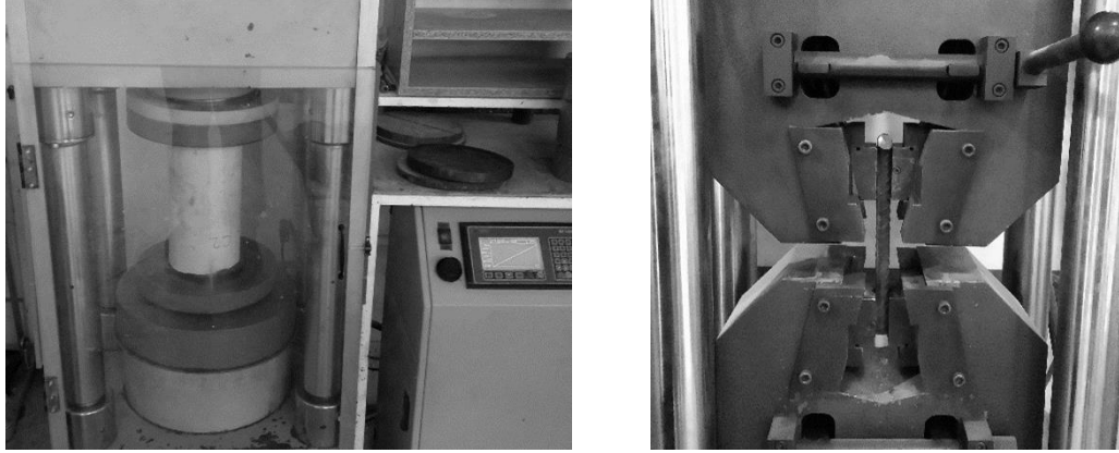
(a) Beton presi
