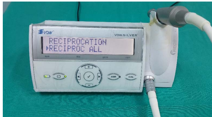
Resim 28. “Reciproc ALL” modundaki VDW Silver Reciproc endodontik motor
