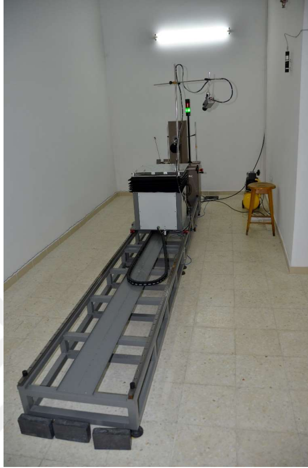
Figure 3.4 Hopewell Designs, Inc., G10 Gamma Beam Irradiator( 137 Cs) and Radiometric Bench ( http://nukbilimler.ankara.edu.tr/kalibrasyon-ve-olcum-laboratuvari/-2019 )
