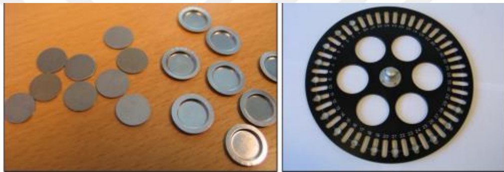
Figure 3.22 Sample discs and cups (planchettes) are shown on the left. On the right a sample carrousel (sometimes referred to as “turntable”) is shown
