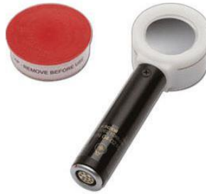
Şekil 3.12 10X6-6M Radcal iyon odası ( http://radcal.com/10x6-6m-mammography-ion-chamber , 2019)
