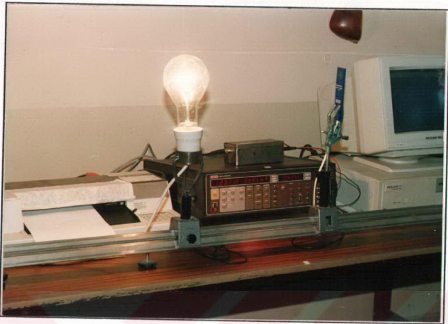
Figure 5.1-4 Experimental set up for measuring the density of sensitizing centers by the CV method.
