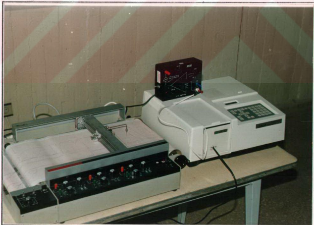
Figure 5.3-3 Experimental set up to measure the band gap of a photoconductor.
