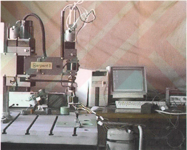
Figure 4.13 The photograph of Serpent 1 with PLC
