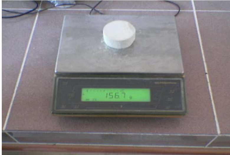
Figure 3.3. A balance of adequate capacity, capable of determining the mass of specimen to an accuracy of 0.01%.
