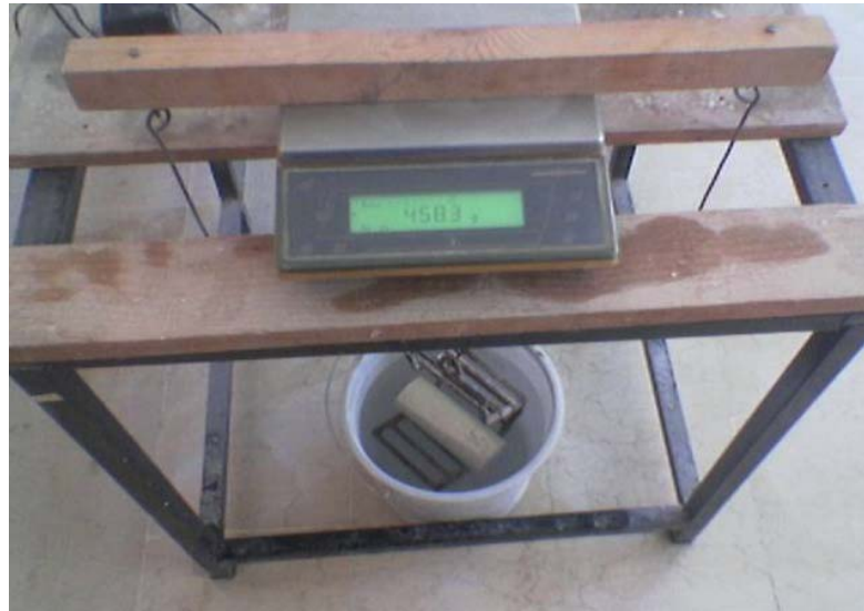
Figure 3.2. An apparatus used for calculating the volume by using the Archimedes' law
