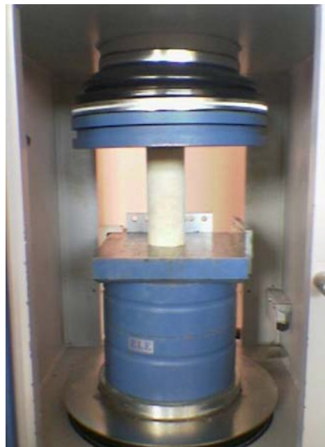
Figure 3.8. A suitable machine shall be used for applying and measuring axial load to the specimen
