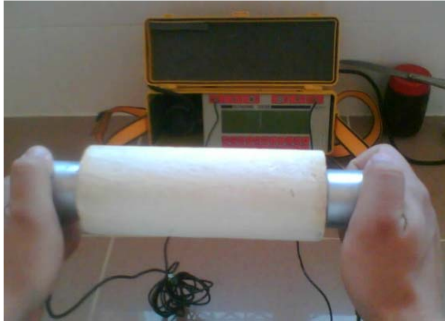
Figure 3.5c. The ultrasonic velocity test performed on core specimen for uniaxial compression test
