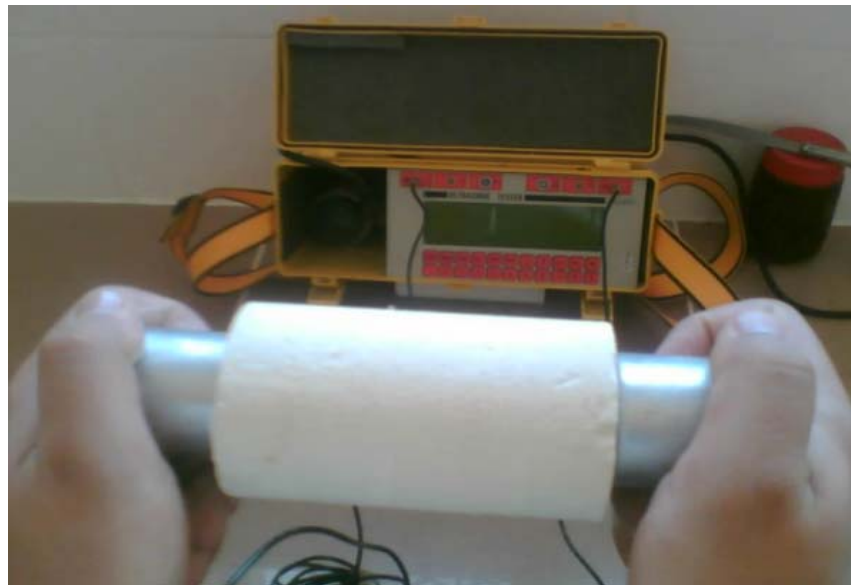
Figure 3.5b. The ultrasonic velocity test performed on core specimen for direct shear test.
