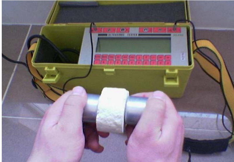
Figure 3.5a. The ultrasonic velocity test performed on core specimen for Brazillian test.
