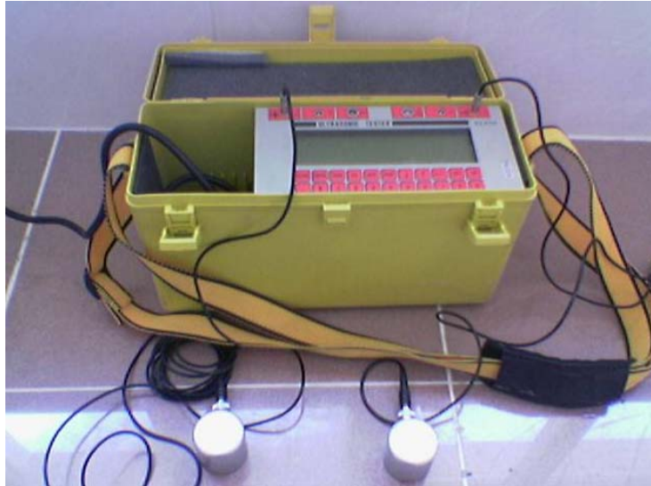
Figure 3.4. Ultrasonic velocity test equipment.
