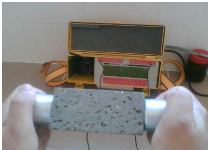
Figure 3.5b. The ultrasonic velocity test performed on block specimen for direct shear test
