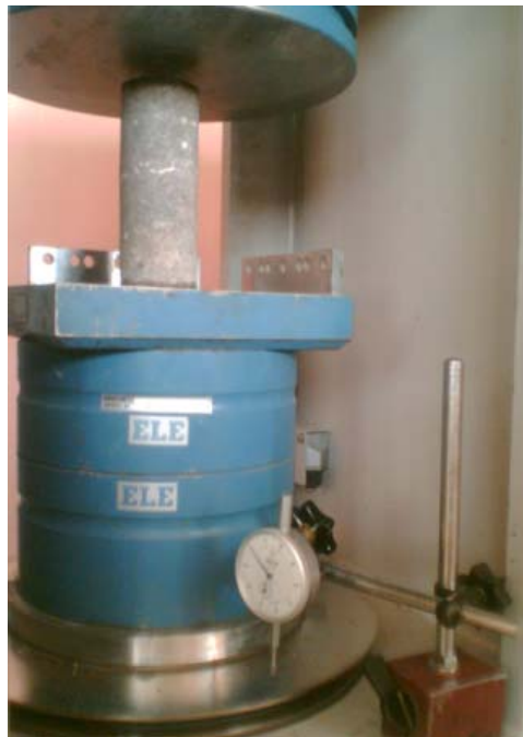
Figure 3.8. A suitable machine shall be used for applying and measuring axial load to the specimen
