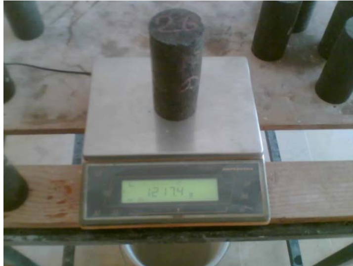
Figure 3.3. A balance of adequate capacity, capable of determining the mass of specimen to an accuracy of 0.01%.
