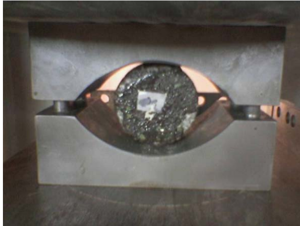
Figure 3.6a. The suggested apparatus for Brazil Test (ISRM 1981)
