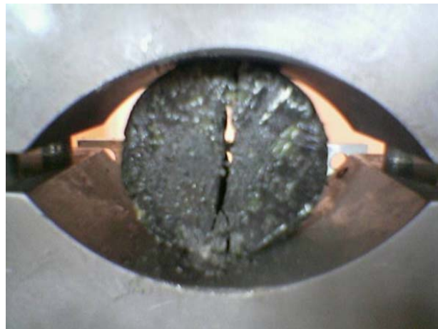
Figure 3.6b. The suggested apparatus for Brazil Test (ISRM 1981)
