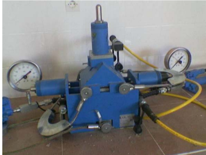
Figure 3.12. Arrangement for laboratory direct shear test.
