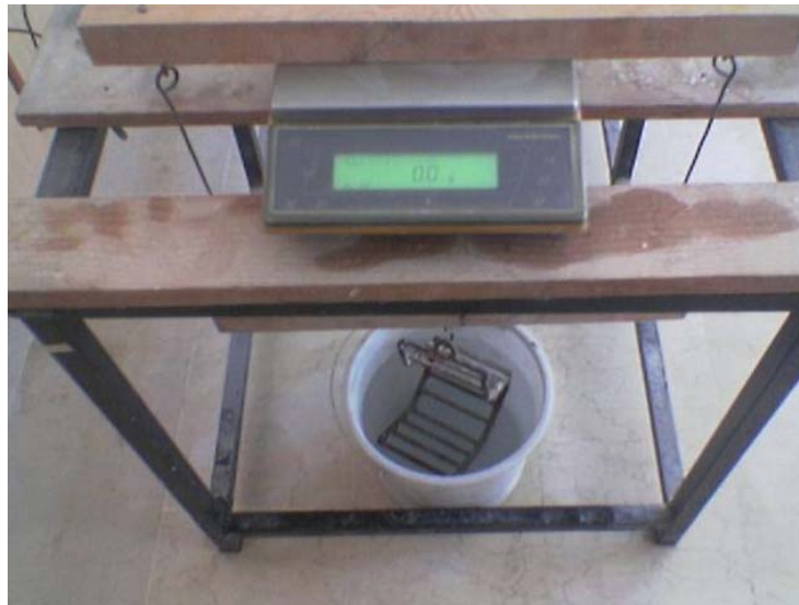
Figure 3.2. An apparatus used for calculating the volume by using the archimed's law
