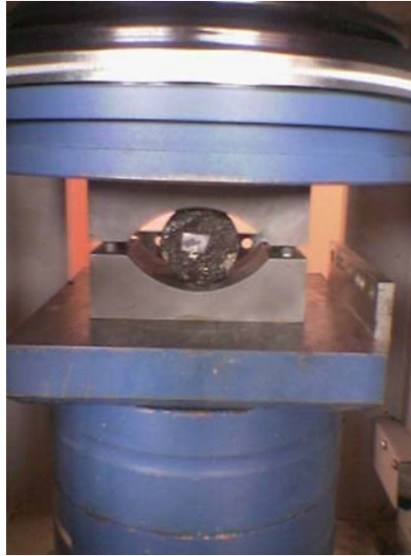
Figure 3.7. A suitable machine for applying and measuring compressive loads to the specimen
