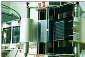
Figure 3.1 A roll-base laminating system
