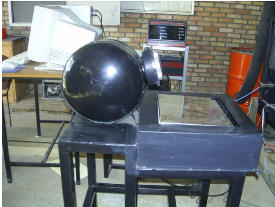
Figure 3.10: The Fuel Flow Measuring System
