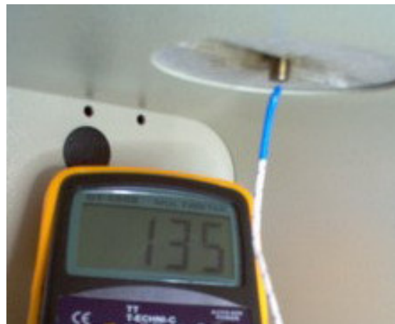
Figure 4.10 Temperature measurement on the end point of designed spinneret hole
