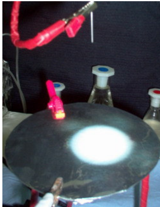
Figure 5.3 Formation of electrospun TPU fibers onto collector
