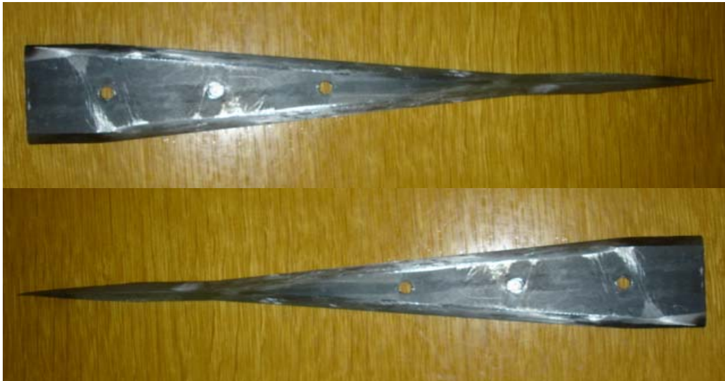
Fig. 5.22 Wedge Tools Used Experimental Setup (Fig. 5.24) \alpha=25 , \beta=9 where thickness is 2mm
