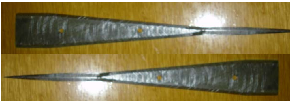
Fig.5.16. Wedge Tools Used Experimental Setup \alpha=25 , \beta=9 and Thickness 2mm
