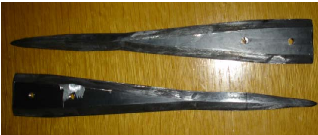
Fig. 5.24 Wedge Tools Used Experimental Setup (Fig. 5.23) \alpha=30 , \beta=7 where thickness is 4mm
