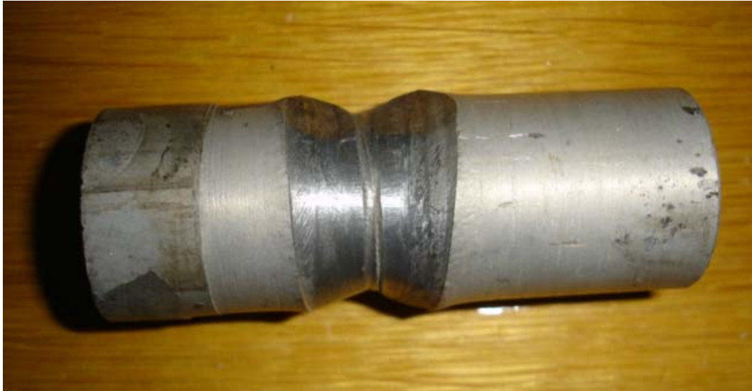
Fig. 5.27 Photographs of Aluminium Obtained from Wedges in Fig. 5.24 with Heating the Workpieces to 400 C
