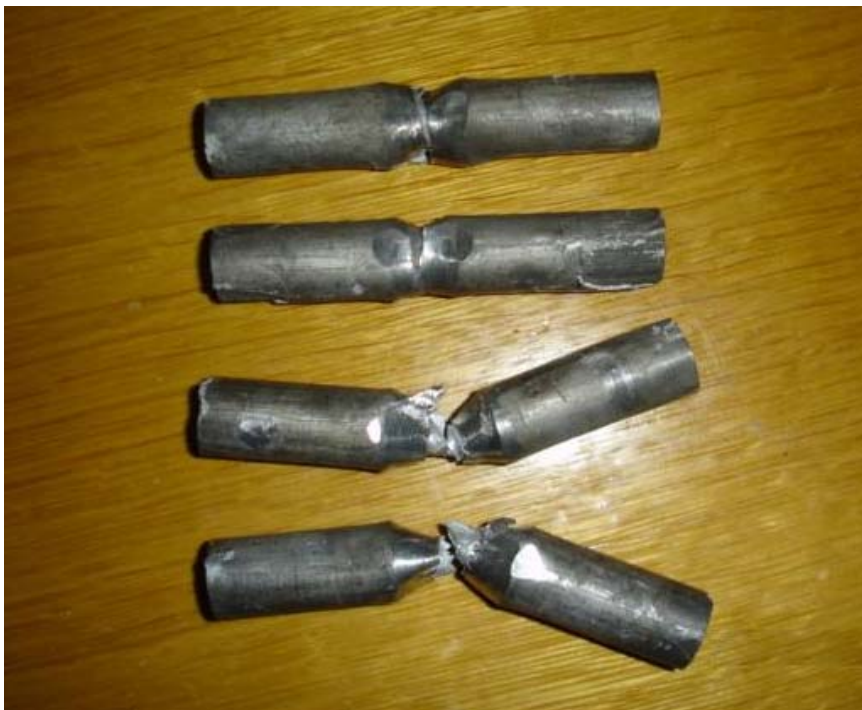
Fig. 5.26 Photographs of Aluminium Obtained from Wedges in Fig. 5.24 with Heating the Workpieces to 400 C
