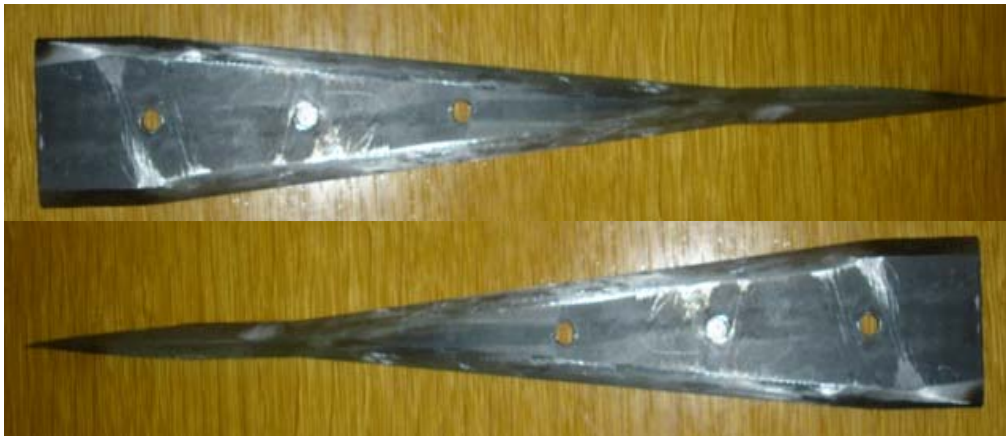
Fig.5.15. Wedge Tools Used Experimental Setup \alpha=20 , \beta=7 and Thickness 2mm
