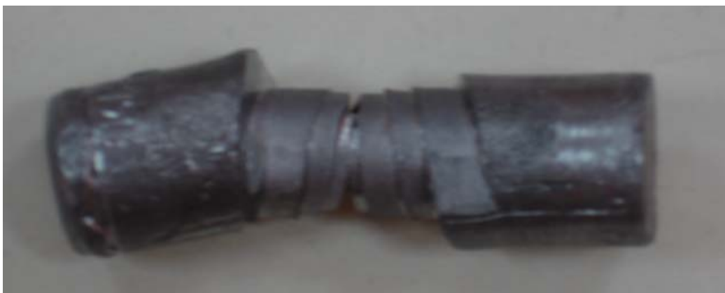
Fig.5.8 Workpiece Failure Obtained from the Wedge in Figure 5.7.
