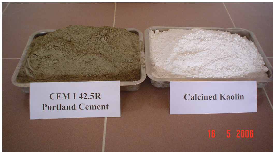
Figure A1 Photographic view of Portland cement and calcined kaolin (in the form of metakaolin)
