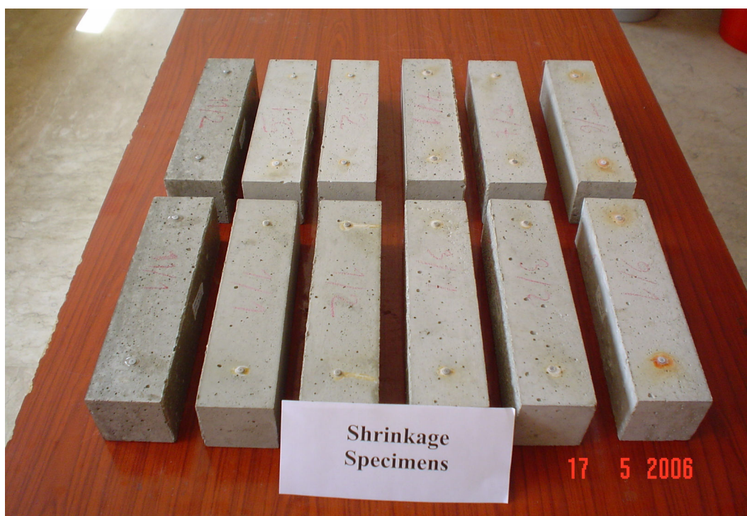
Figure A2 Photographic view of shrinkage specimens
