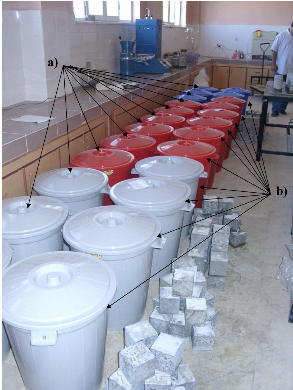
Figure A4 Photographic view of \text{Na}_2\text{SO}_4 solution tanks which were utilized for a) continuous exposure b) cyclic exposure
