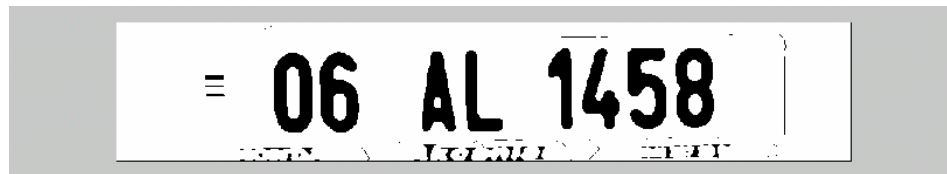
Figure 4.8: Plate image after filtering and dilation operation
