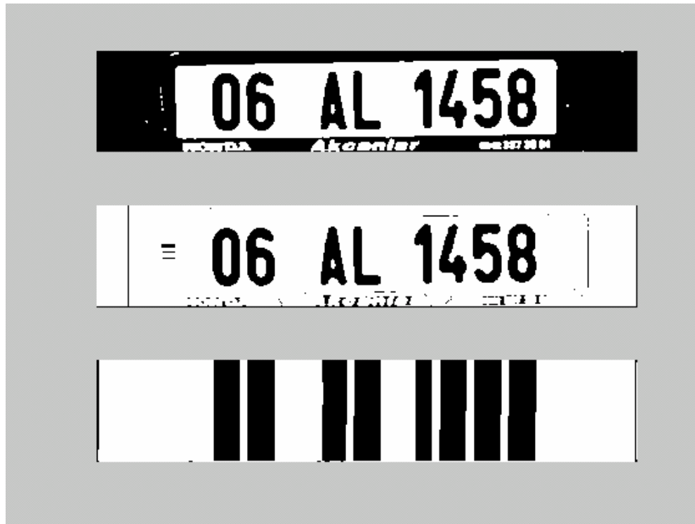
Figure 4.9: Plate images showing segmentation
