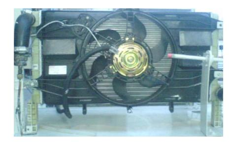
Figure 3.9 Photograph of air-cooled absorber
