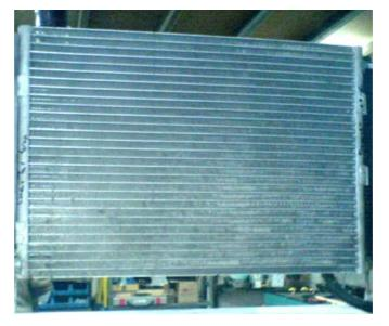
Figure 3.11 Photograph of air-cooled condenser
