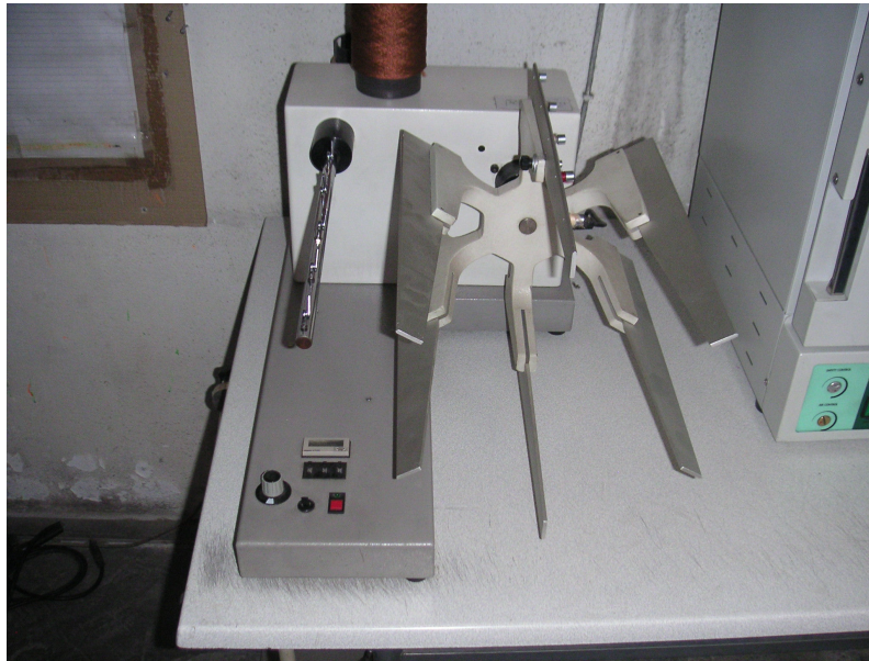
Figure 5.2 The wrap reel
