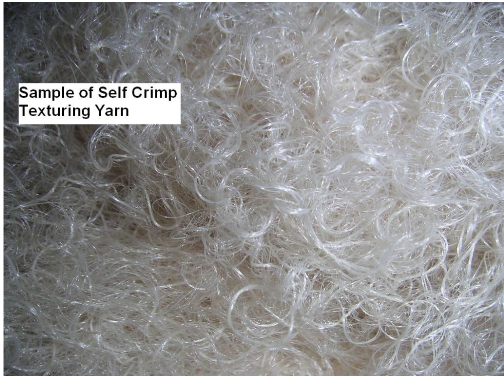
Figure 4.26 The Self-Crimp FYS yarn samples
