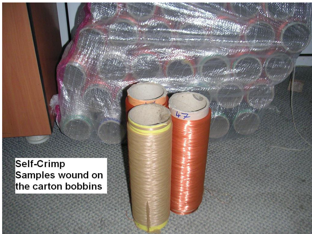
Figure 4.27 The Self-Crimp texturing yarns wind on the carton bobbins
