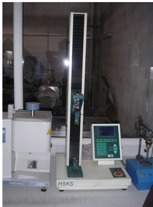
Figure 5.3 Yarn Tensile Strength Tester
