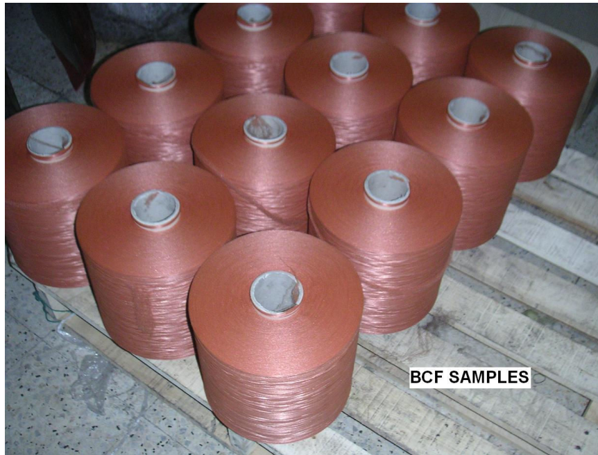
Figure 1.1 The BCF Carpet Yarn Bobbins
