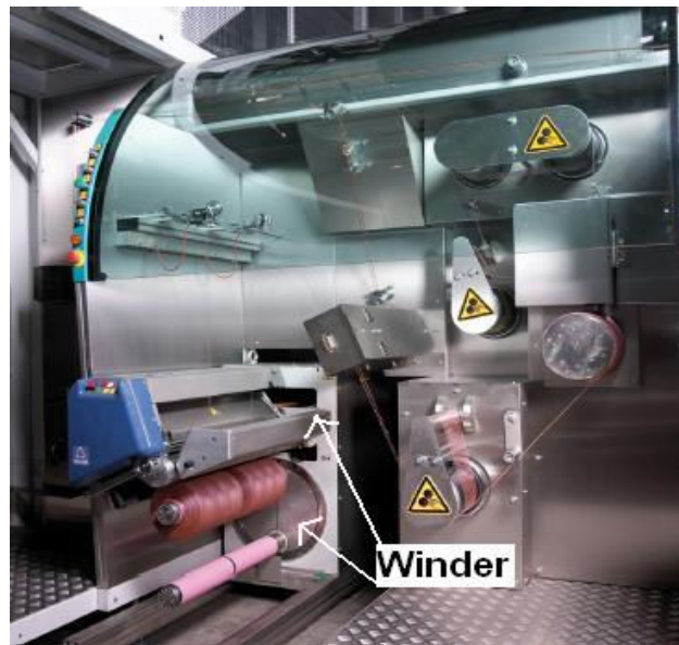
Figure 2.16 The winding and drafting units of SML BCF machine [31]
