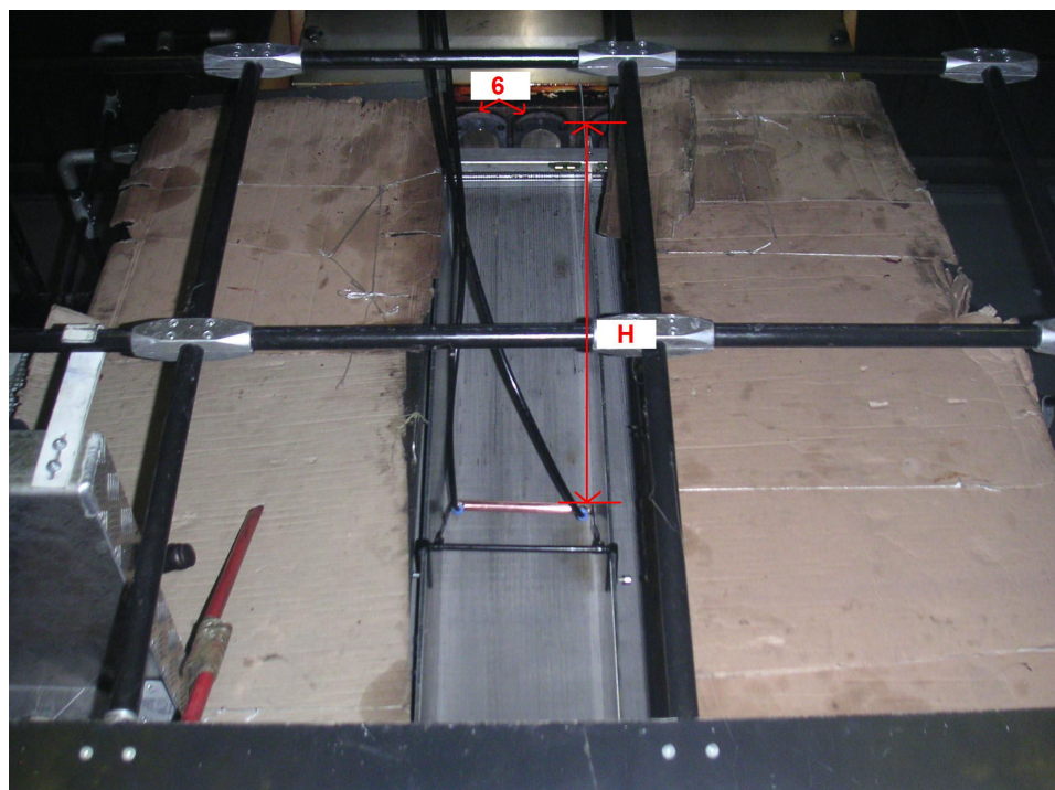
Figure 4.17 The distance of the local cooling apparatus
