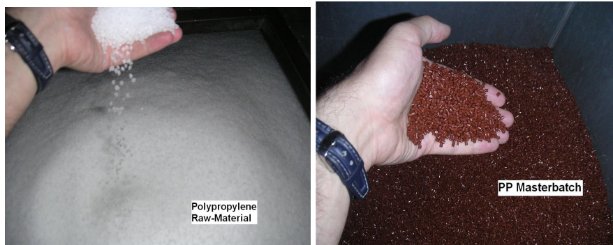
Figure 2.5 %100 Polypropylene and masterbatch chips
