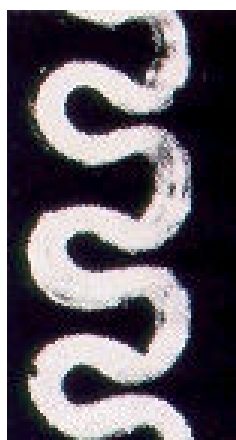
Figure 3.10 The Knit-de knit yarn [36]
