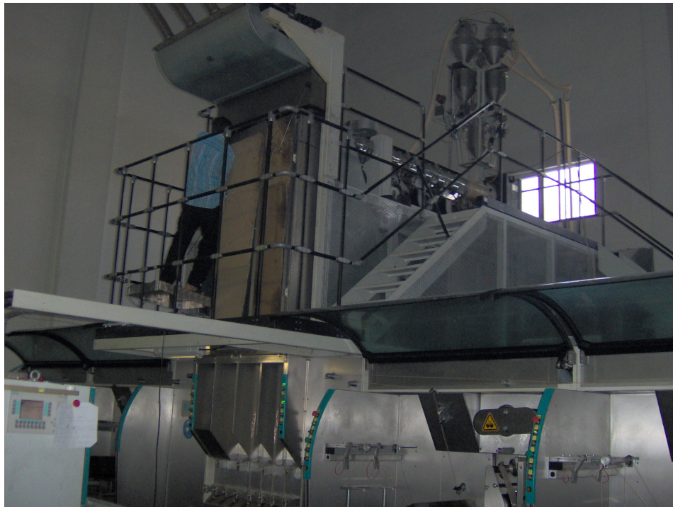
Figure 4.1 The BCF Spinning Machine made by SML
