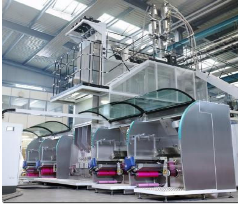
Figure 2.4 The SML BCF production machine [31].
