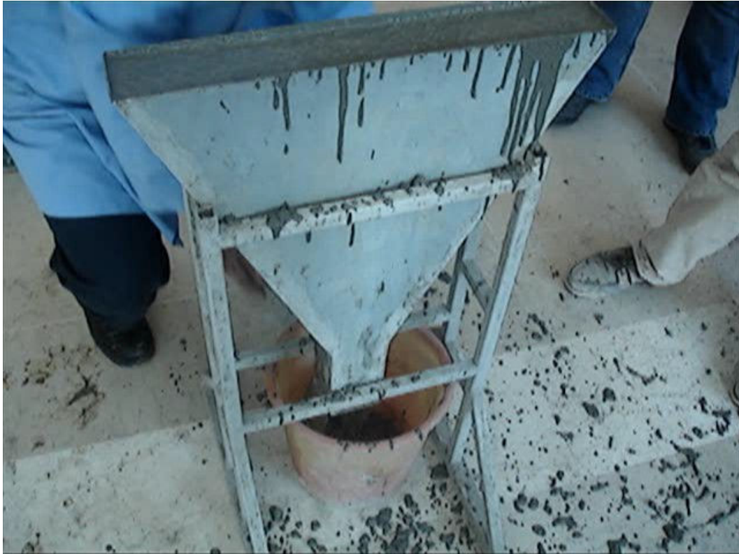
Figure 3.3 Photographic view of V-funnel flow time measurement
