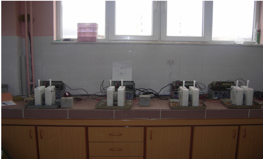
Figure 3.10 Rapid chloride permeability test
