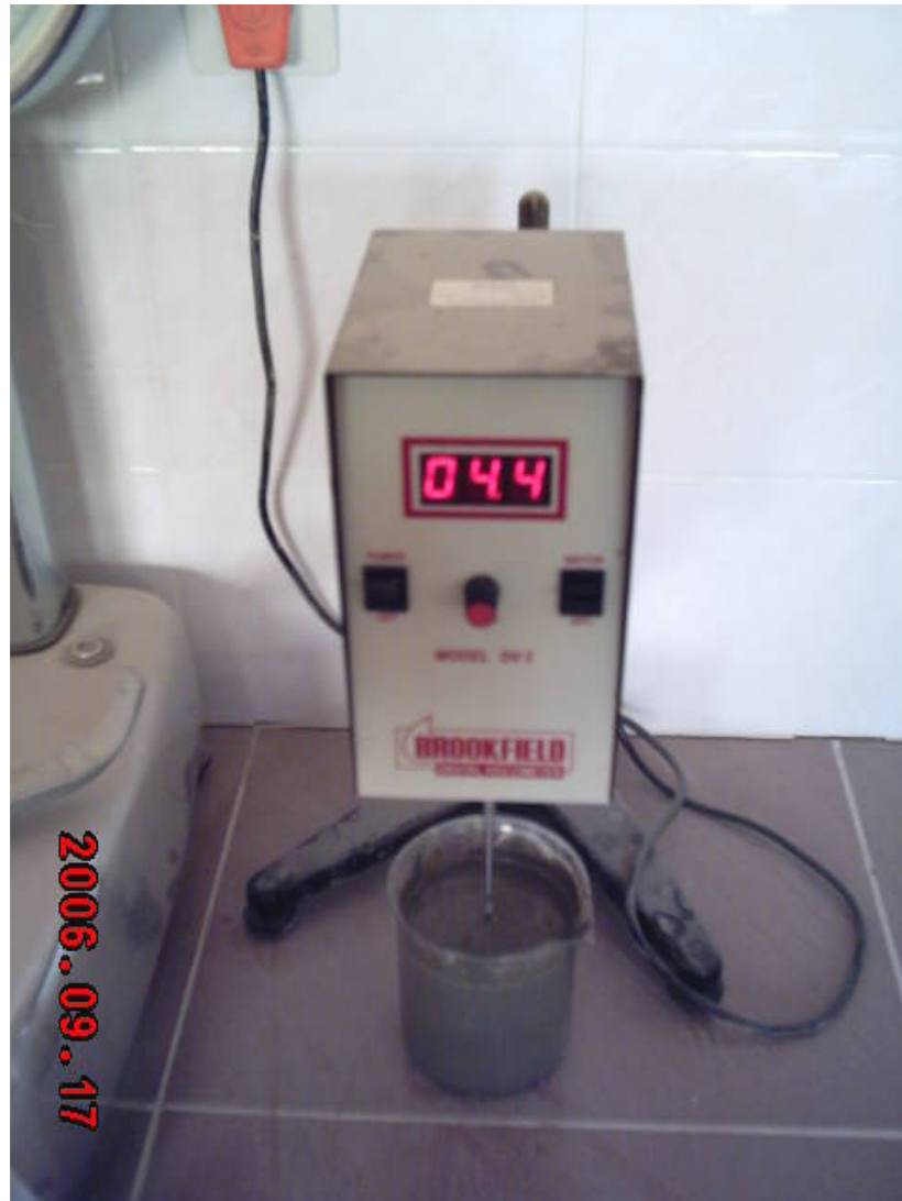
Figure 3.6 Photographic view of viscosity test apparatus and measuring of viscosity
