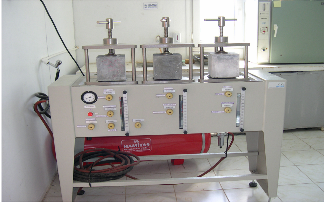
Figure 3.14 Photographic view of water permeability test equipment
