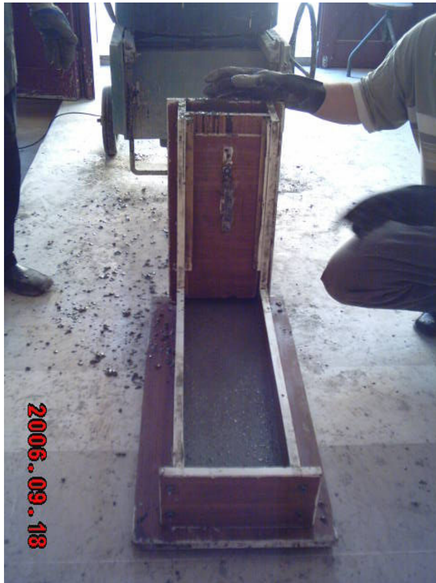
Figure 3.4 Photographic view of L-box apparatus and testing procedure
