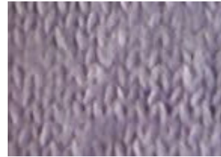
Figure 3.11 Knitted fabric with S twisted and Z twisted yarn
