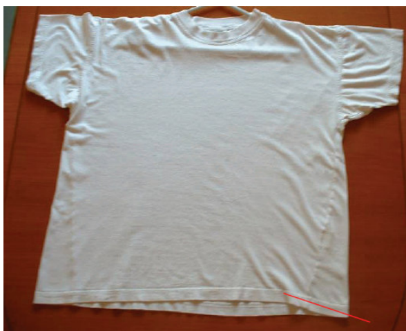
Figure 4.3 Distortion of side seam after laundering
