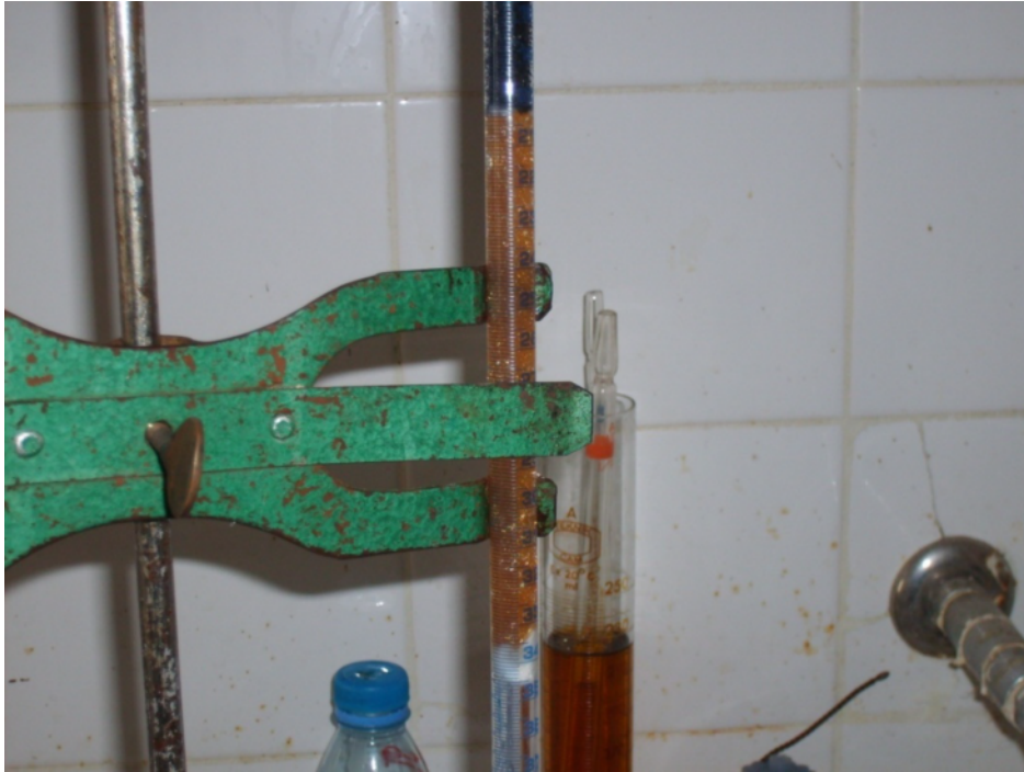
Figure 2.6. Activated carbon column
