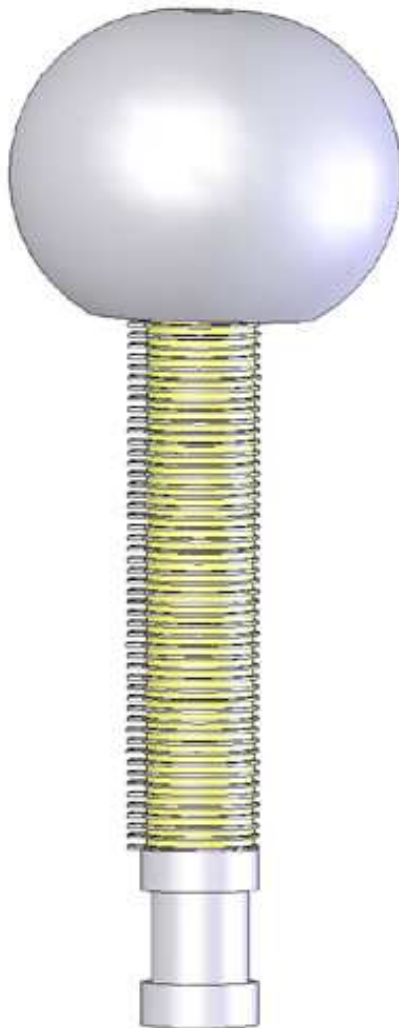
Figure 3.21: Accelerator tube as attached to the HV sphere. A connection flange or a "T" flange could be used at the end depending on the use of vacuum system
