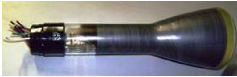
Figure 3.16: RCD 3RP1 cathode ray tube used as sample particle, electron source in the simulation of the accelerator unit in SIMION 3D (v7.0).
