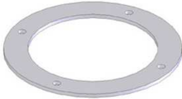
Figure 3.4: Two connection HDPE rings for fixing the support column and the lower high voltage terminal. Dimensions are shown on technical drawings and given in appendix B with Part number 3
