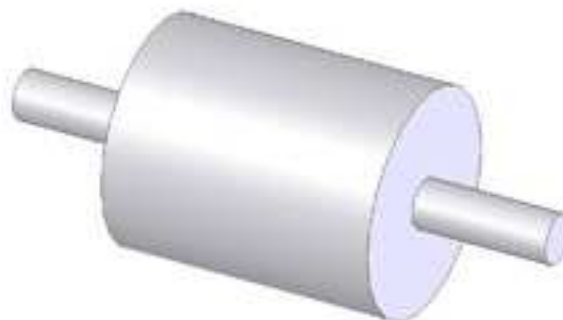
Figure 3.6: Rollers, would be used to rotate the endless belt between the HV and ground terminals. Dimensions are shown on technical drawings and given in appendix B with Part number 5
