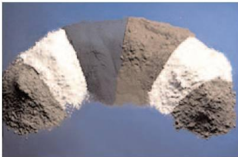
Figure 2.21-Photographic view of supplementary cementitious materials. From left to right, fly ash (Class C), metakaolin (calcined clay), silica fume, fly ash (Class F), slag, and calcined shale. (PCA, 2003)
