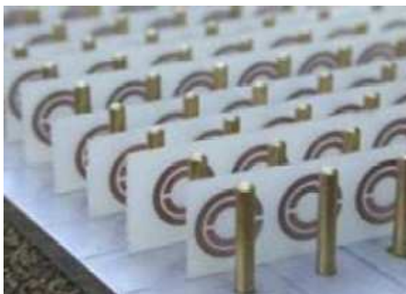
Figure 3.4: First metamaterial comprised of metallic rods and circular split rings.
