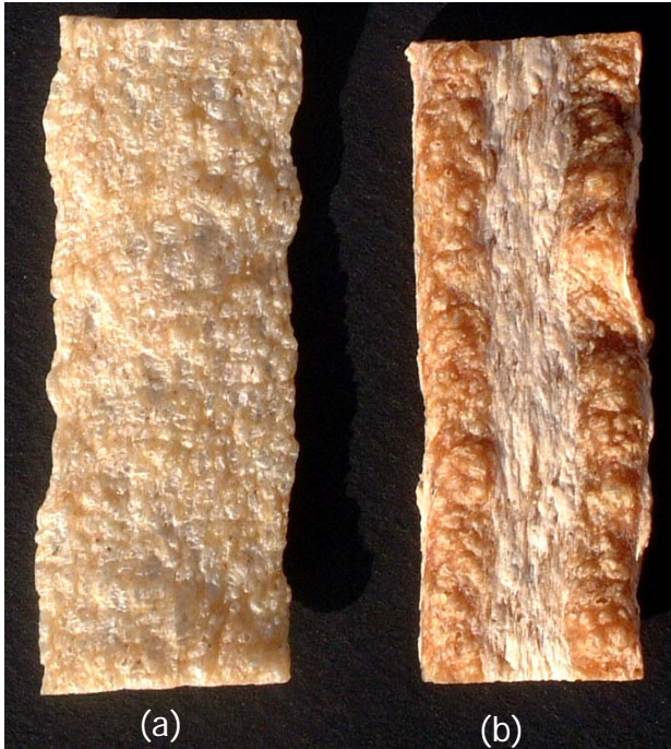
Figure B.15 Images of extrudates produced at 150°C and 175 rpm with different grape pomace level: (a) 0% and (b) 12.7%
