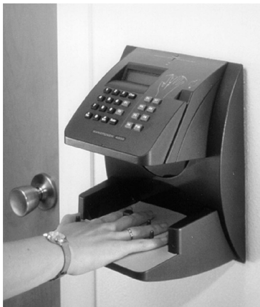
Figure 2.1: A hand recognition system for access control
