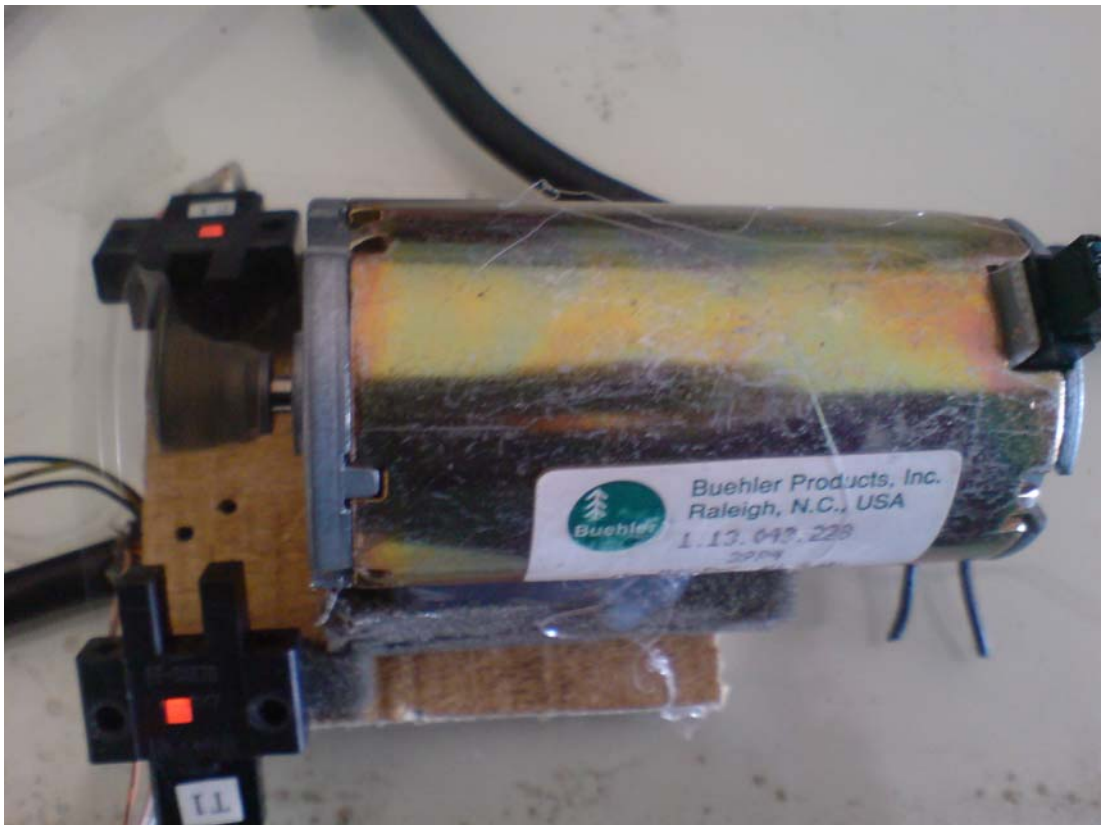
Figure 4.2 T1 and T2 sensors with an electrical engine to simulate the mechanism
