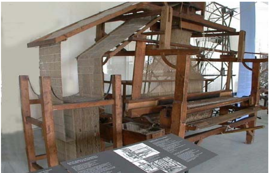
Figure 1.5 Punch card loom
