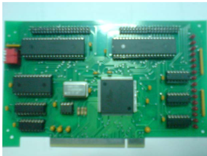
Figure 2.16 Top view of the I/O card after all production steps
