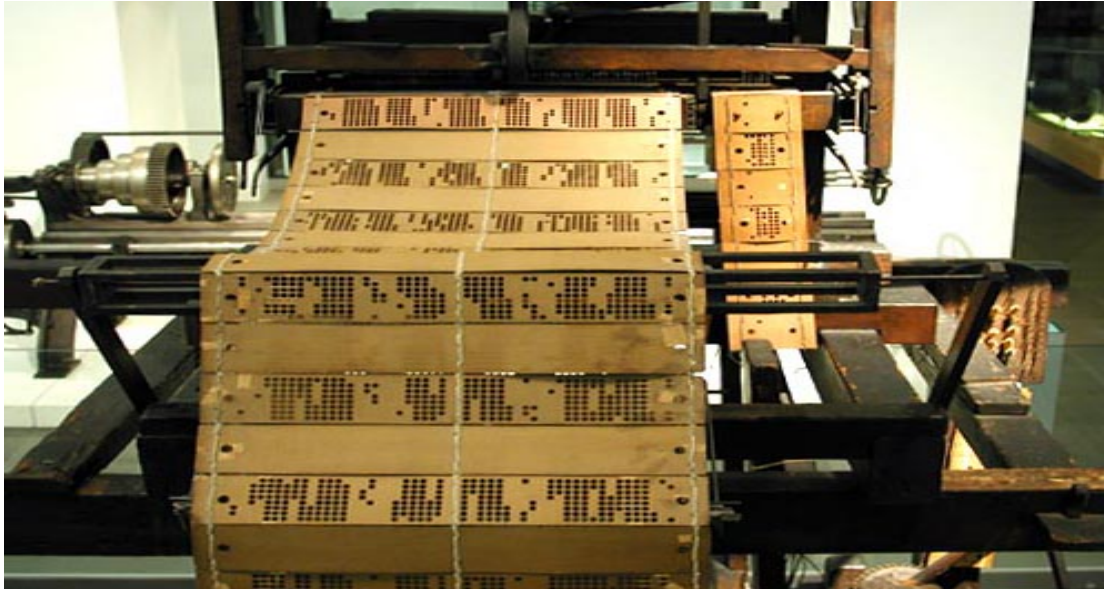
Figure 1.4 Punch card mechanism
