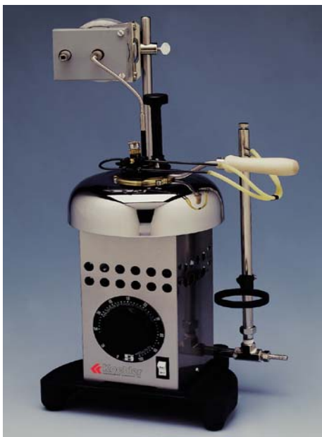
Figure 3.16 K16200 Pensky-Martens closed cup flash tester.
