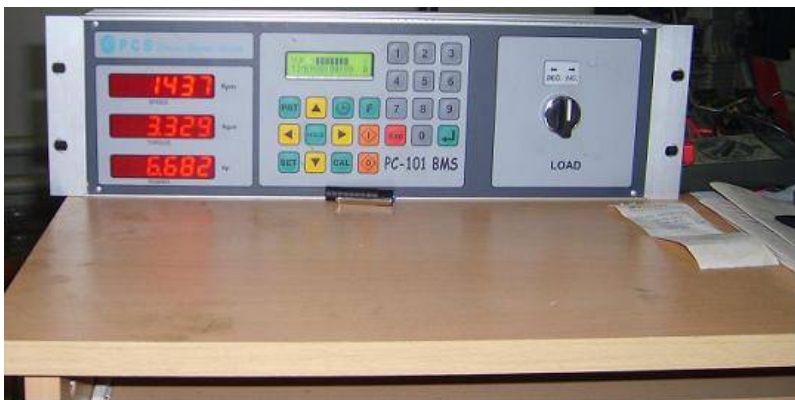
Figure 5.5 Diesel test engine control panel.
