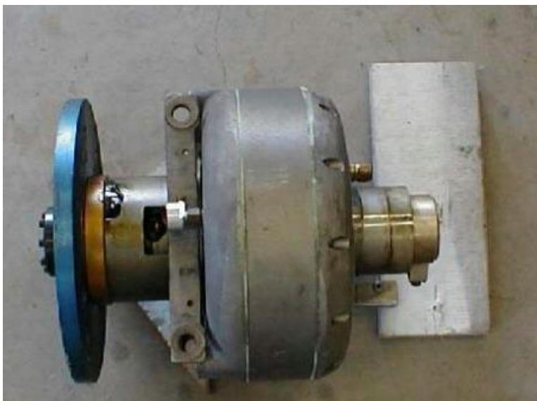
Figure 6.6 Go Power System DA 516 model water brake dynamometer.
