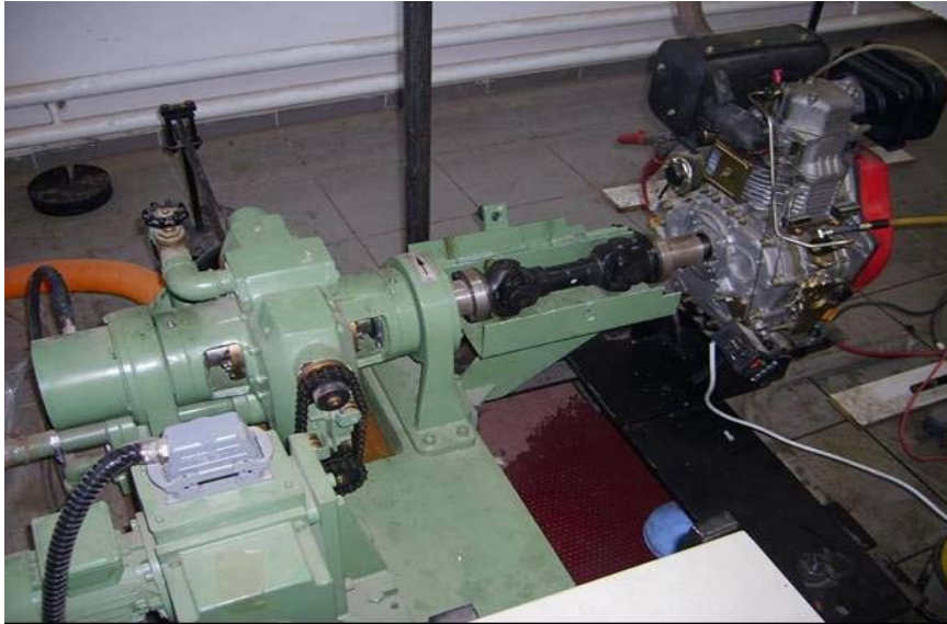
Figure 4.2 Diesel test engine and its dynamometer.
