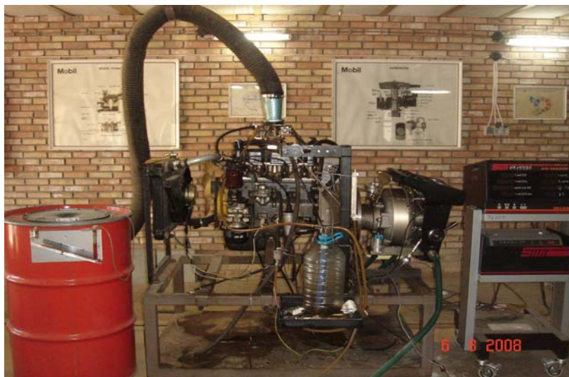
Figure 6.3 Picture of the gasoline (SI) test engine.
