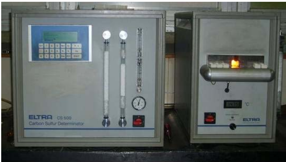
Figure 3.18 Eltra CS500 Carbon/Sulfur determinator.
