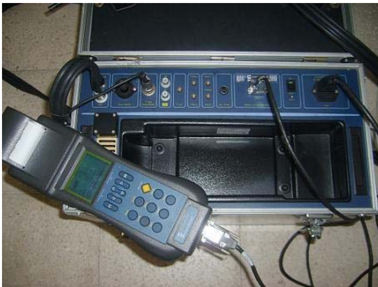
Figure 5.6 Greenline 8000 exhaust analyzing device.
