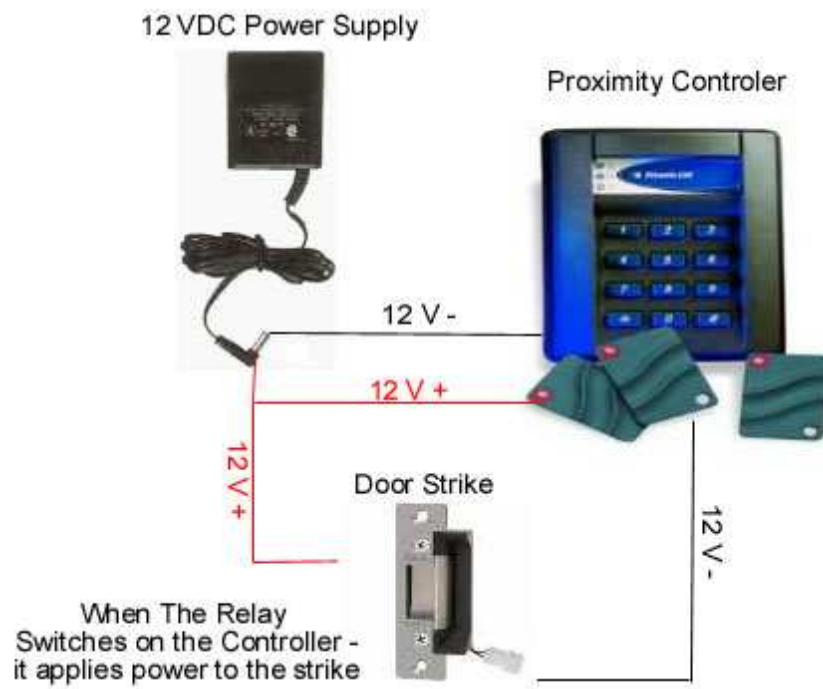
Figure 2.9 Proximity access controllers
