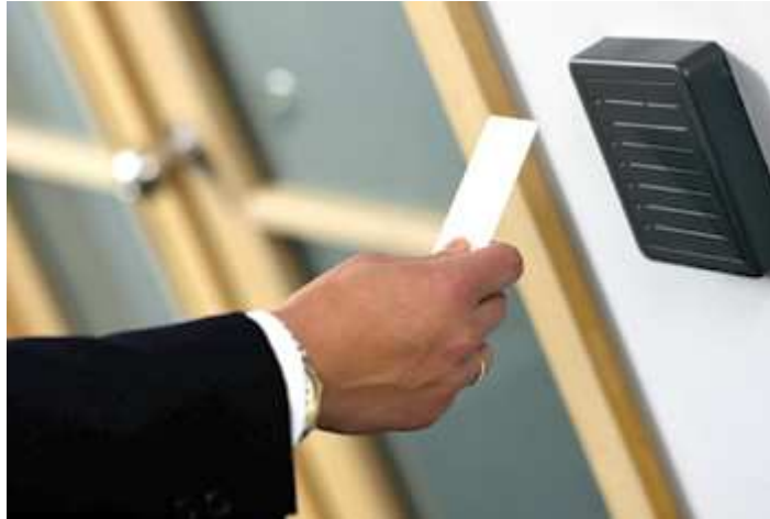
Figure 2.8 Proximity card reader
