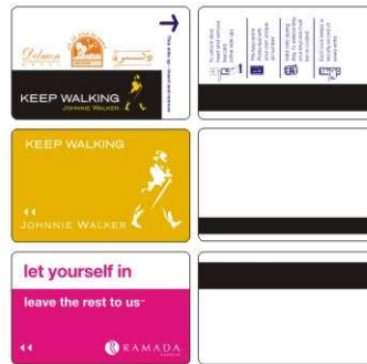
Figure 2.6 Magnetic strip cards
