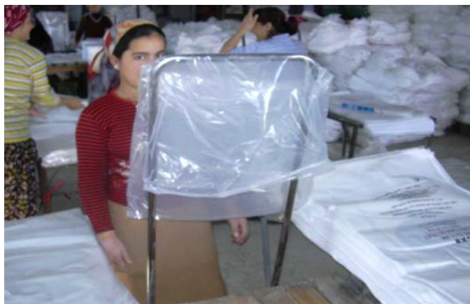
Figure 2.3. Placing the PE sack on the sack inserting platform
