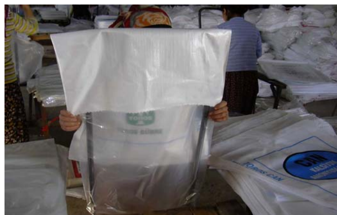
Figure 2.6. Inserting the PP sack onto that of PE
