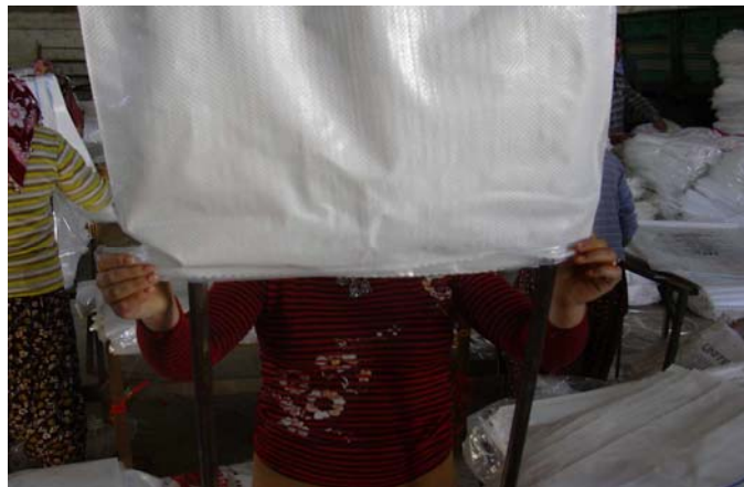
Figure 2.8. Taking off the PE inserted PP sack
