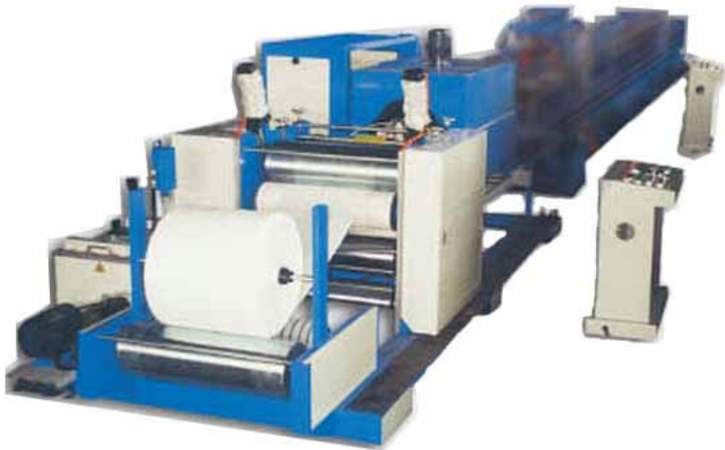
Figure 1.8. PP woven tubular fabric inside lamination machine
