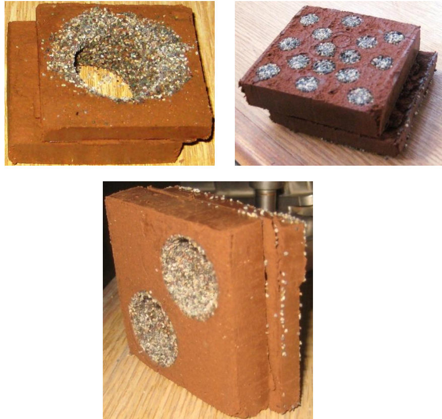
Figure 5.10. The result of direct shear tests of sand-clay mixtures sample photos
