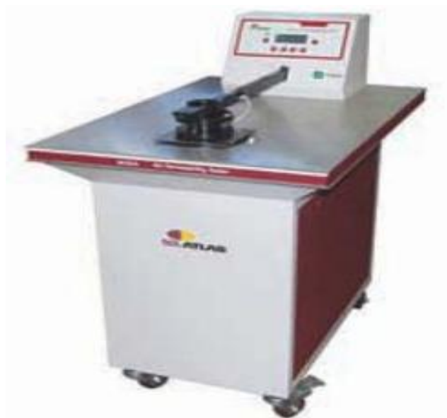
Figure 3.1 M021A SDL ATLAS Air permeability tester [73]
