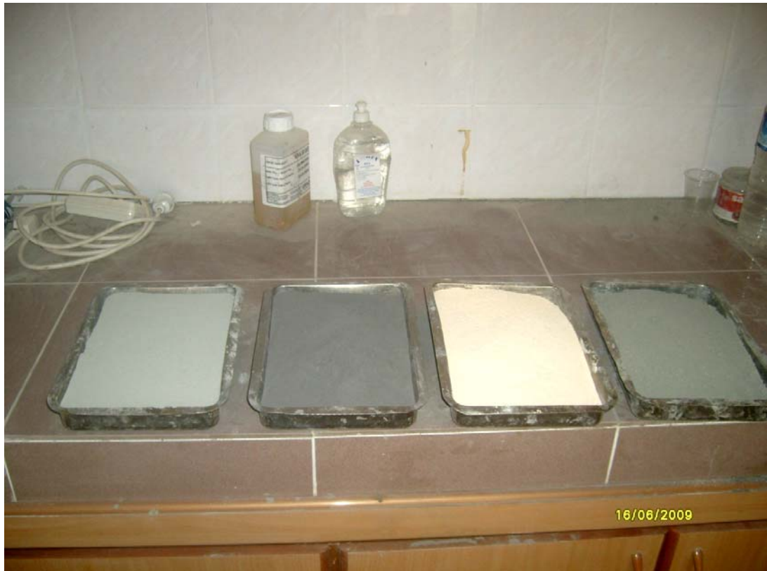
Figure 3.1 Photographic view of mineral admixtures and cement. From left to right; fly ash, limestone filler, marble powder, and portland cement
