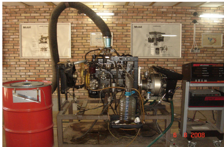
Figure 7.2 Photograph of the SI test engine
