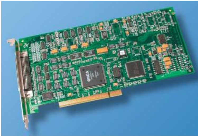
Figure 7.7 DT 304 Data Acquisition Card [180]
