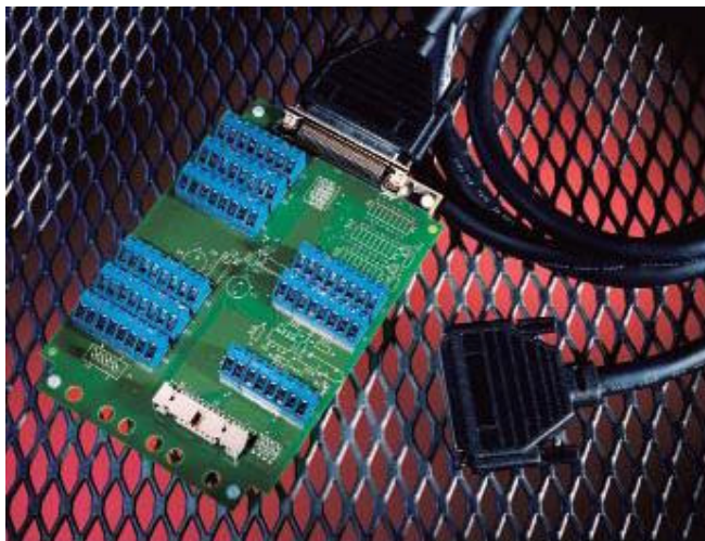
Figure 7.8 Data Translation STP 300 Screw Terminal Panel and EP305 Cable [180]
