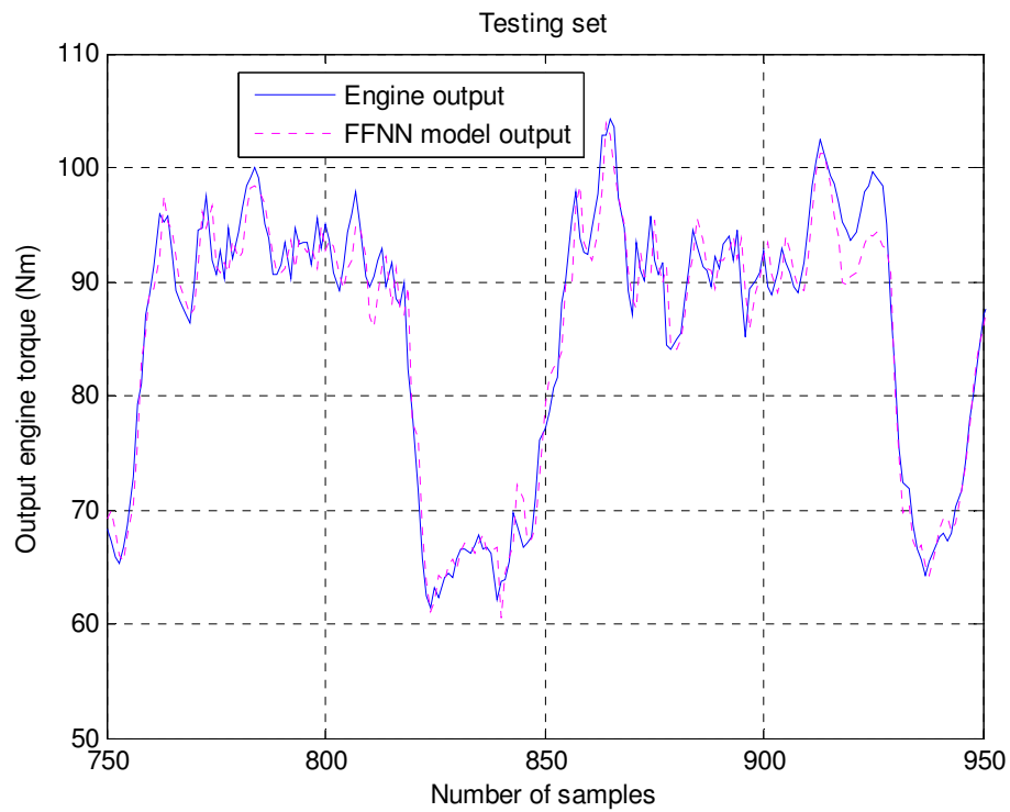
Figure 8.27 Modeling results of the FFNN model with validation of identification results
