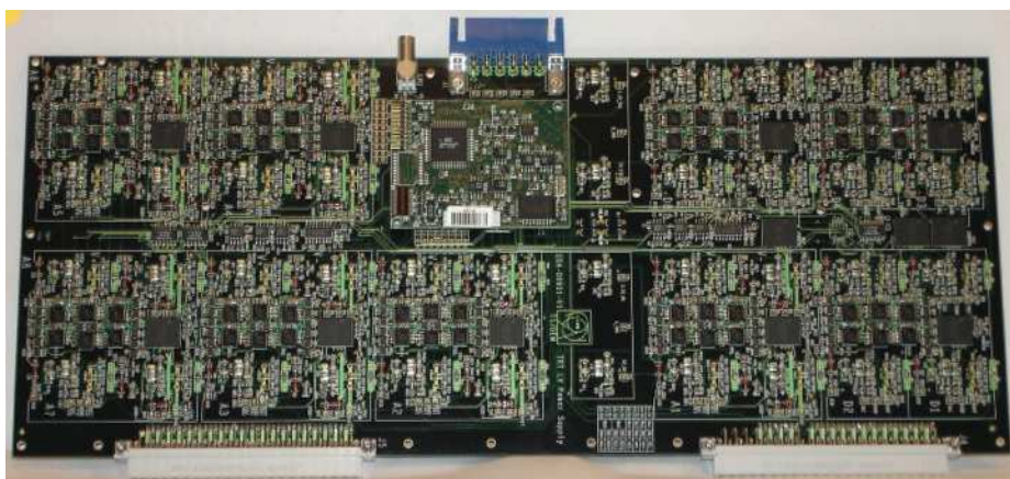
Figure 3.5: Low voltage patch panel board
