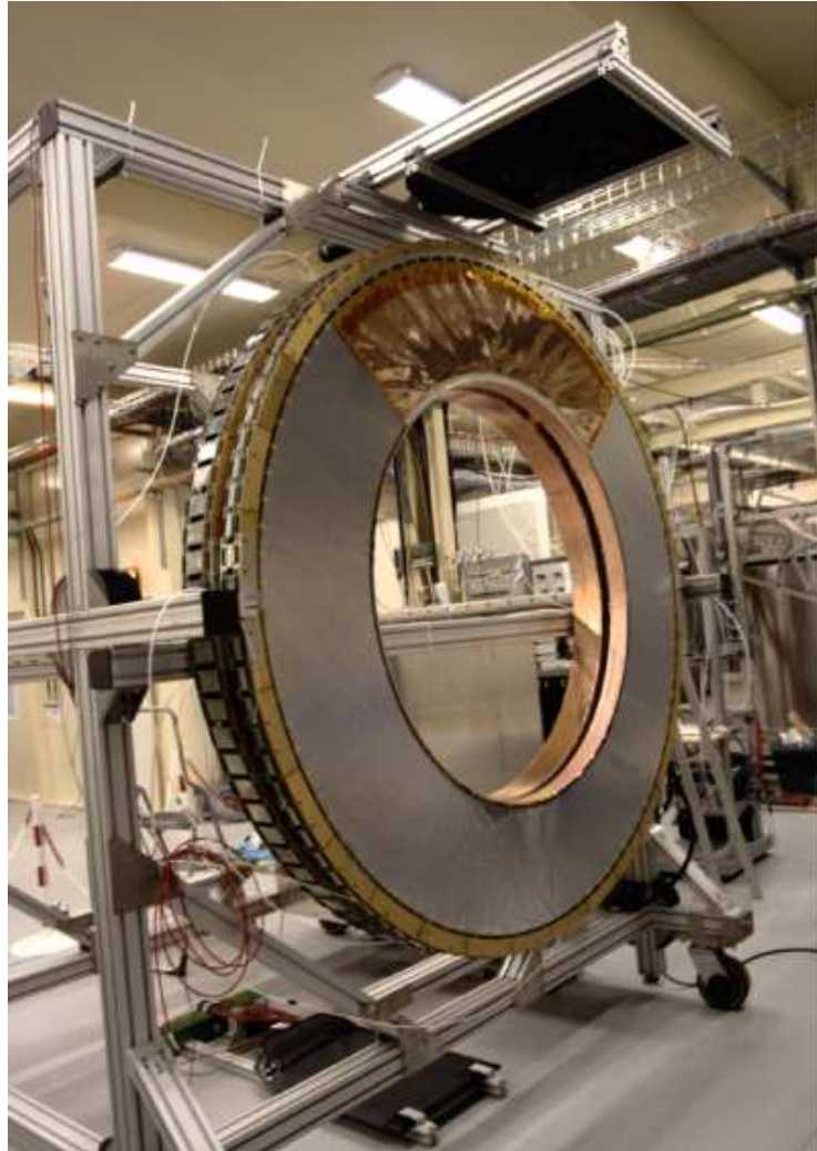
Figure 3.1: System installed in to a Bosch Profile frame. Detector components, readout system (PP2 boxes with electronics, See Section 3.3), cabling is setup in the Bosch profile to provide mobility of the test stand. The system is designed keeping in mind a possibility to use the setup at a test beam for Phase I upgrade studies.
