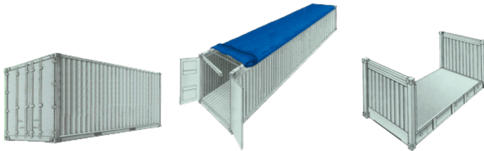
Figure 1.1 Different types of containers (a) General purpose container (b) Open-top container (c) Flat rack
