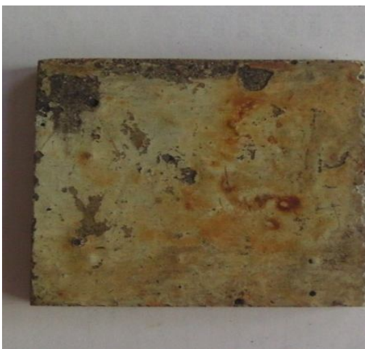
Fig.4. 4 Concrete plate at the bottom part of the shear box
