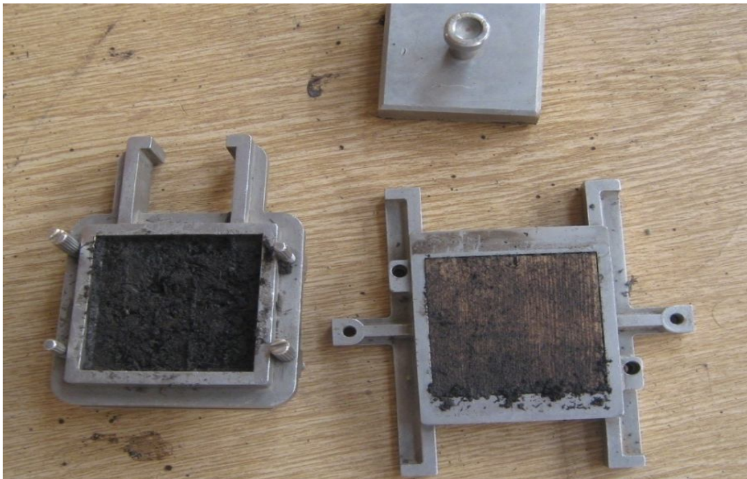
Figure 4. 6 Timber plate at the bottom part of the shear box
