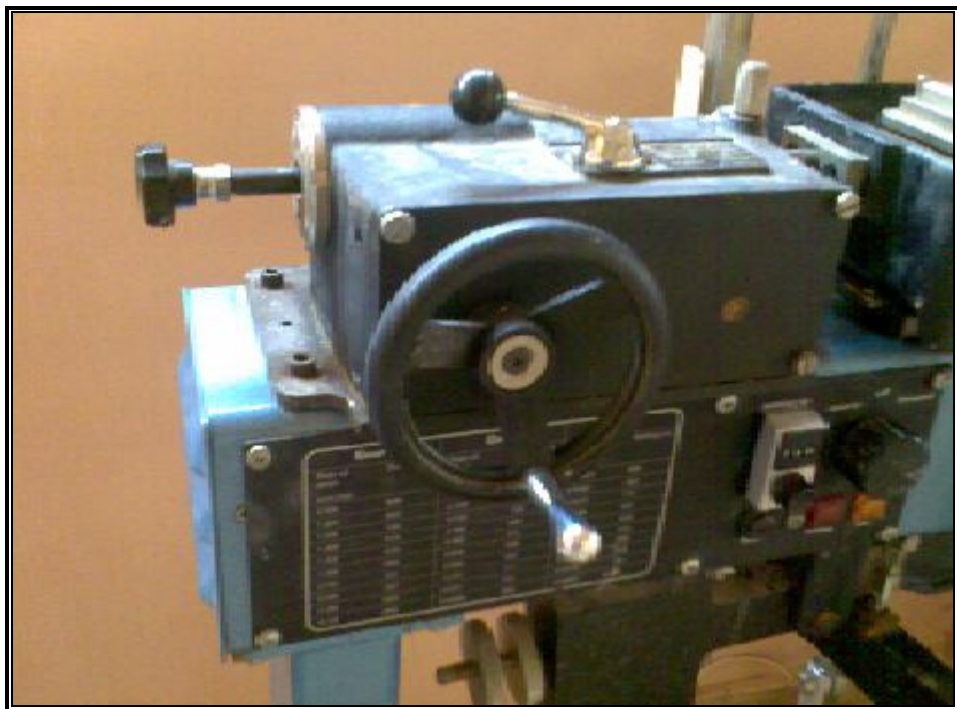
Figure 3.2 Motor and Motor Control Panel of Direct Shear Test
