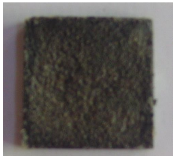
Fig. 4. 5 Rough concrete plate at the bottom part of the shear box
