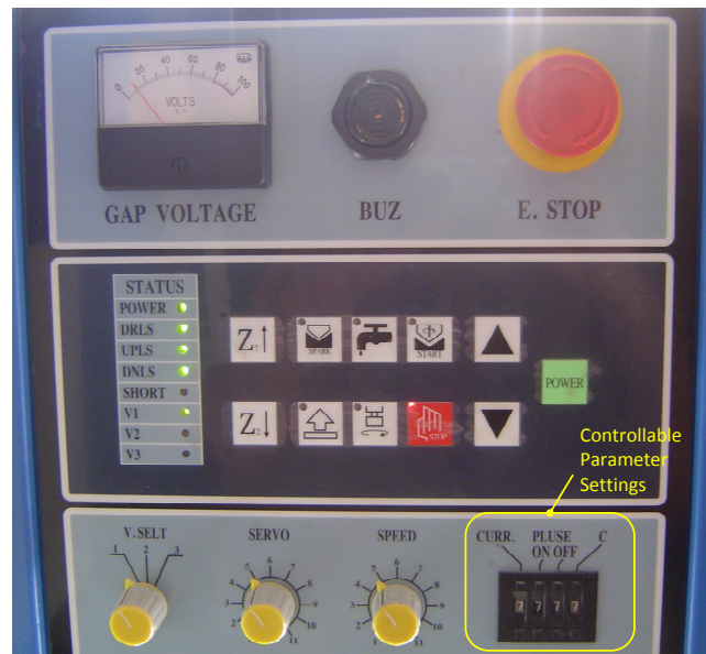
Figure 5.5 Control panel of JS AD-20 EDM machine
