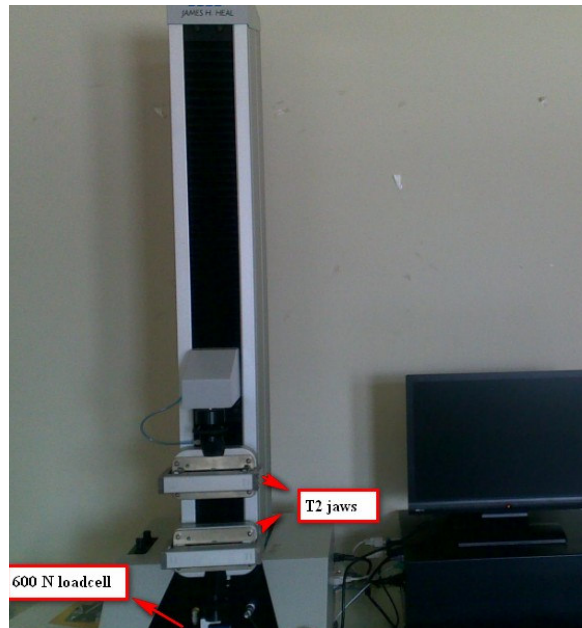
Figure 3.9 Titan universal strength tester 2 with 600N load cell
