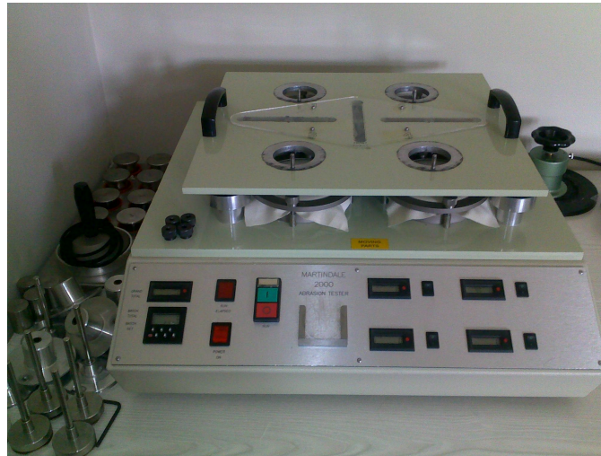
Figure 3.13 Martindale abrasion tester
