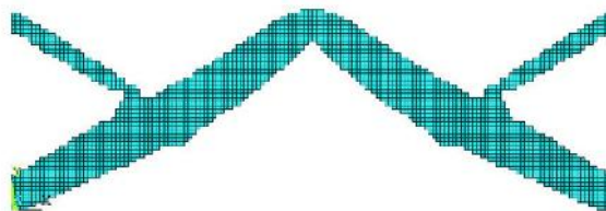
Figure 4.22 The two end fixed beam optimization result under static loading
