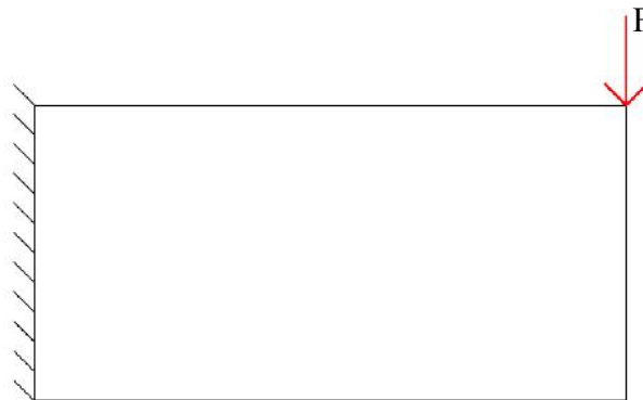
Figure 4.31 Right – top loaded cantilever beam under static loading
