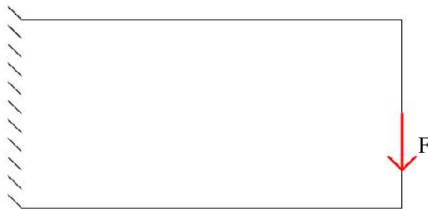
Figure 4.16 The cantilever beam under static loading
