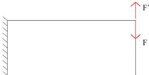
Figure 4.33 Right – top loaded cantilever beam under fatigue loading
