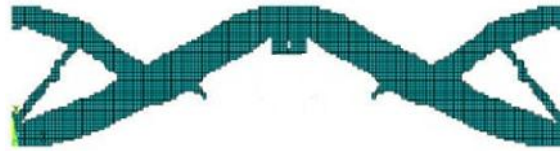
Figure 4.10 Optimization result of top – centre loaded design under fatigue loading
