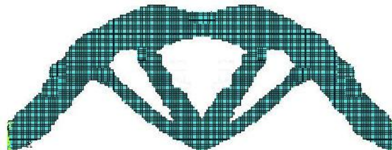
Figure 4.5 Optimization result under fatigue loading for bottom – centre loaded design
