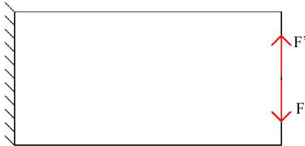
Figure 4.18 The cantilever beam under fatigue loading
