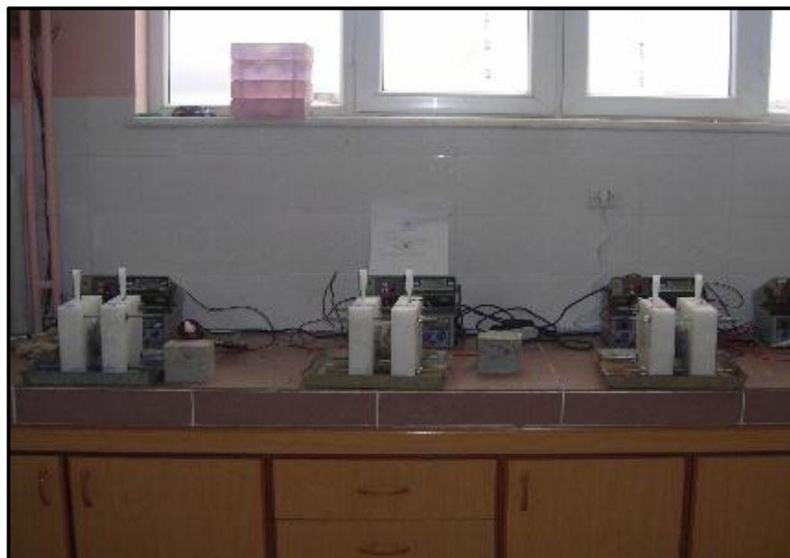
Figure 3.8 Rapid chloride permeability tests
