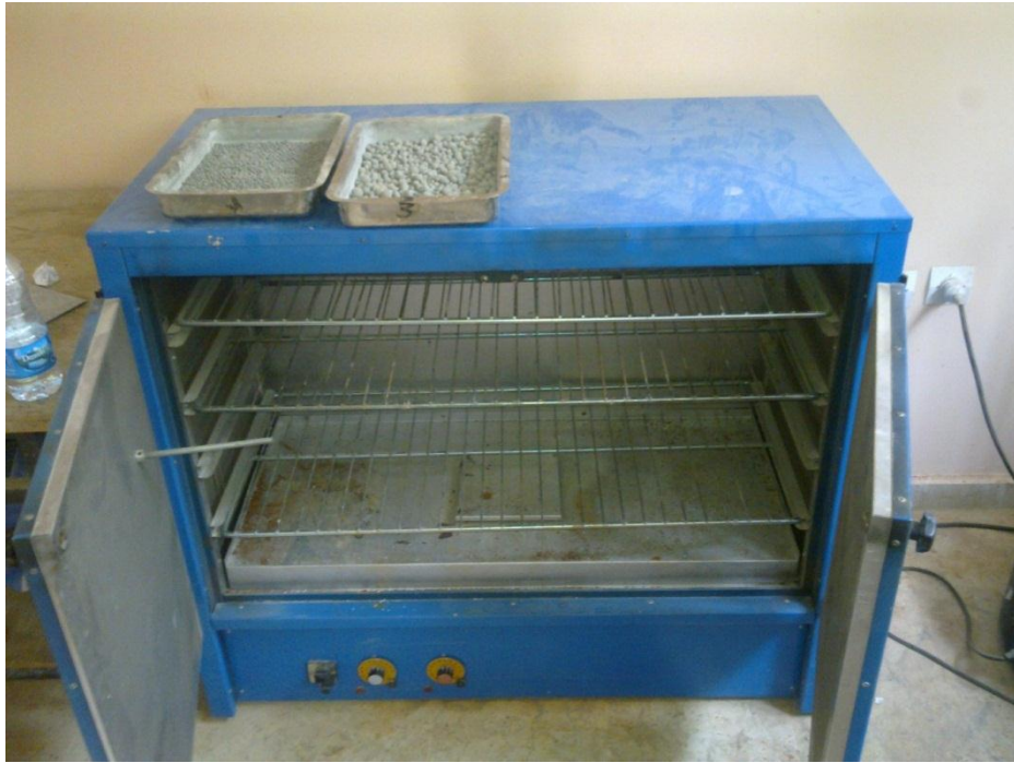
Figure A3 Photographic view of dried LWA in an oven
