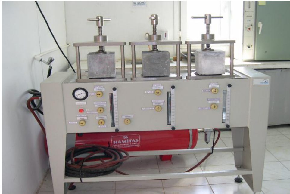
Figure 3.6 Water permeability test set up
