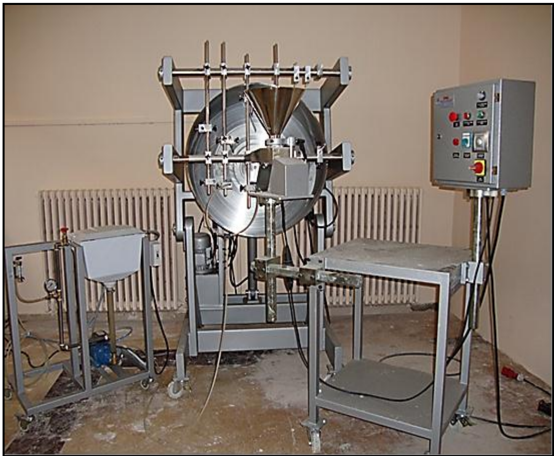
Figure 3.1 The general view of the pelletization disc
