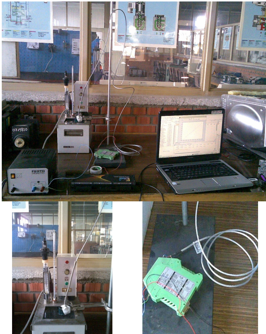
Figure 3.16 PT100 Calibration Process from the Workplace
