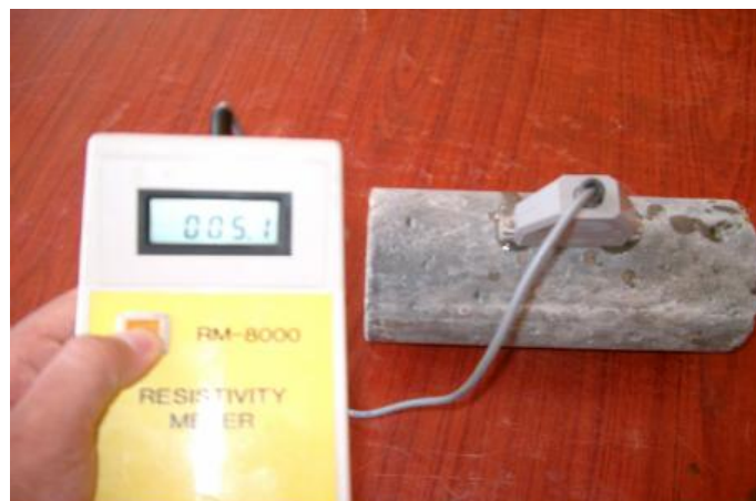
Figure 3.7 Photographic view of the ER test device
