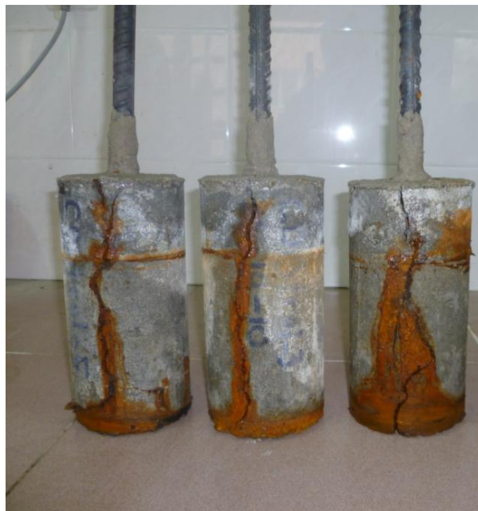
Figure 3.3 Typical corrosion specimens after finishing ACT
