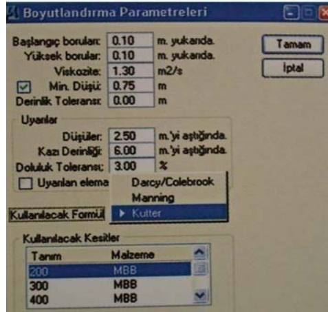
Figure 6.18 Stormwater pipe parameters in MsKanal program [57].
