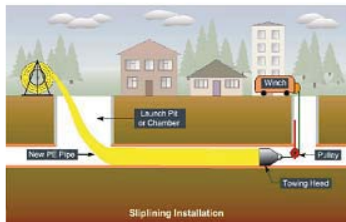
Figure 3.5 Slip lining installation [40].
