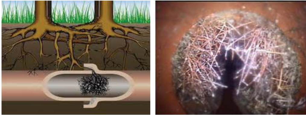
Figure 2.2 Root intrusions in sewer pipe [7, 8].
