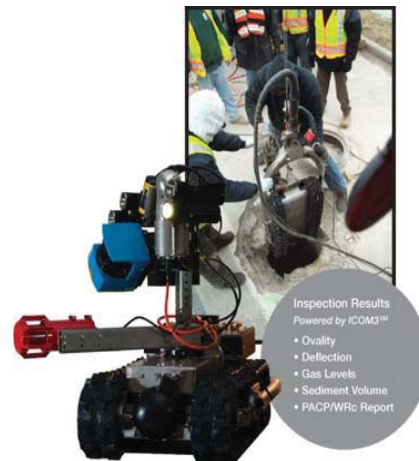
Figure 3.15 Large diameter pipe inspection systems [44].
