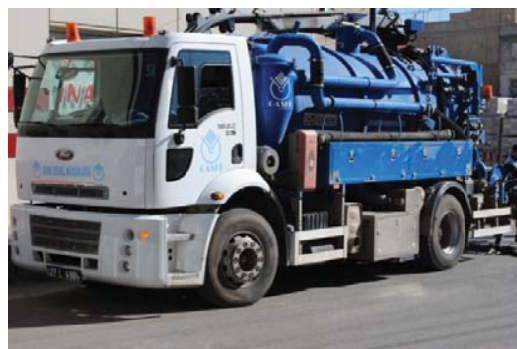
Figure 3.23 Shows flushing jet wagon.
