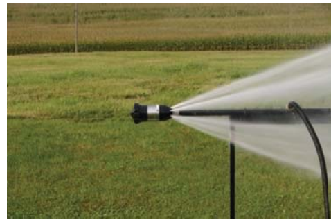
Figure 3.22 Flushing nozzles in sewer system [48].
