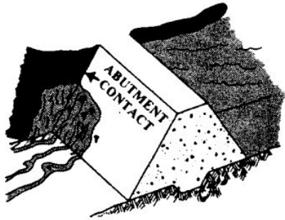
Figure 2-18 Seepage Exiting at Abutment Contact
