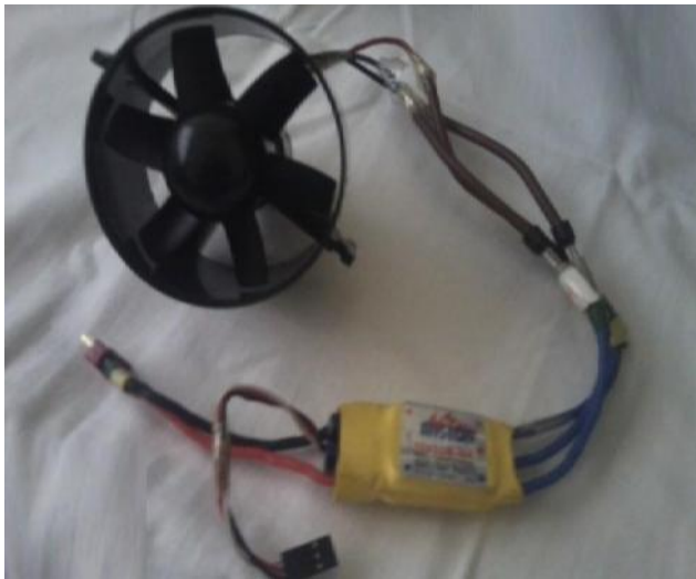
Figure 5. 24 Duct Fan Systems
