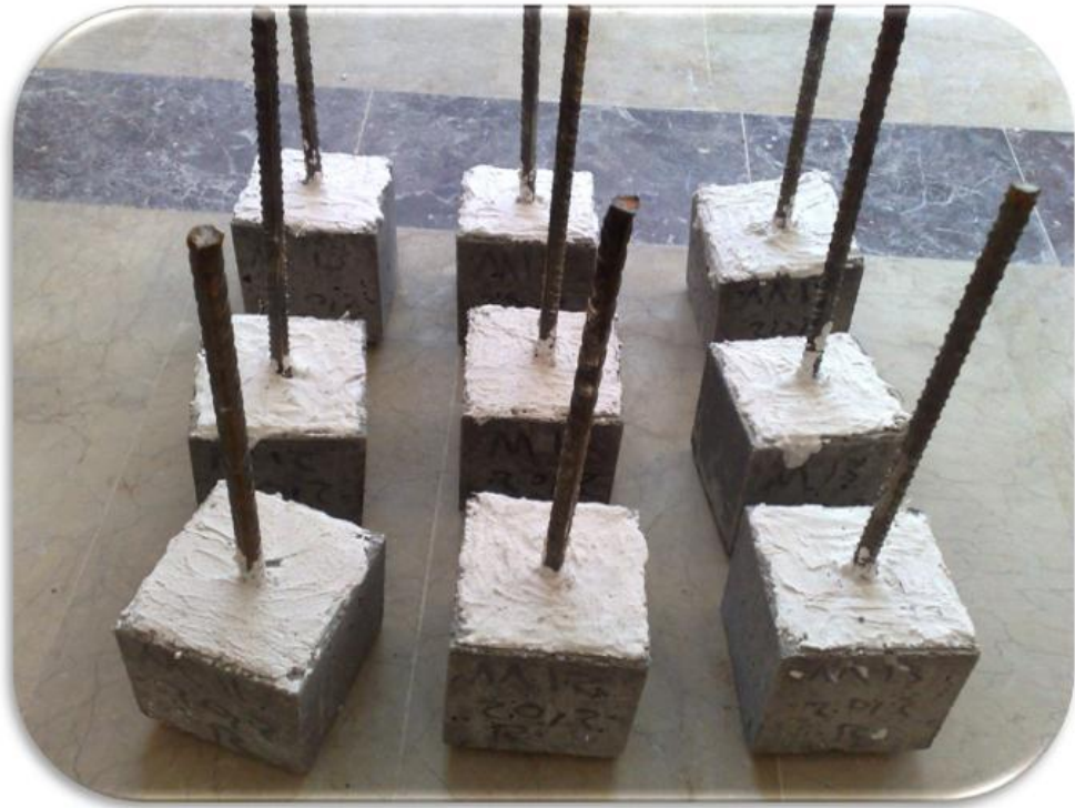
Figure A.11 Pull out specimens before testing for plain and steel fibers mixes
