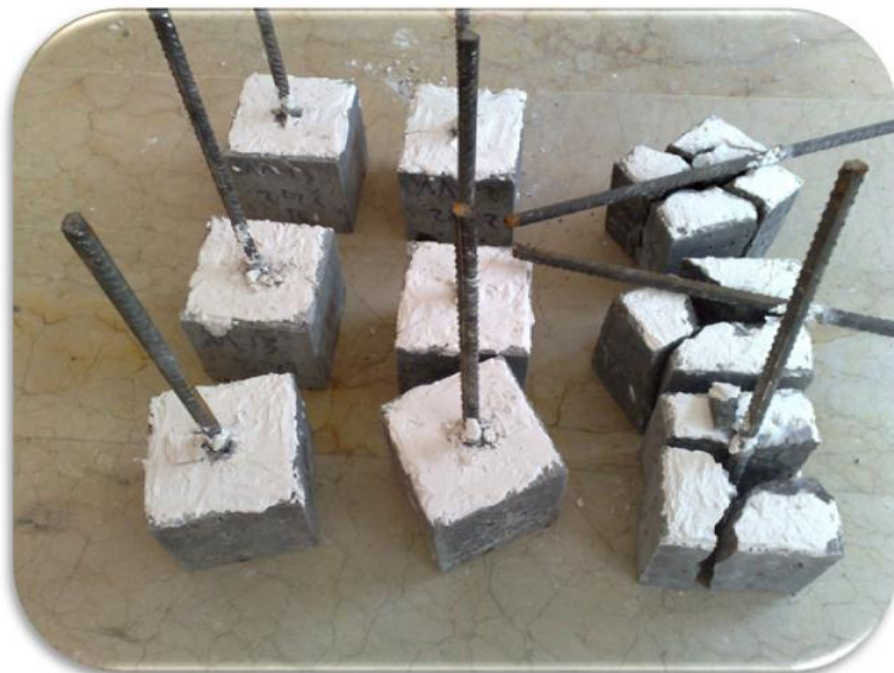
Figure A.12 Pull out specimens after testing for plain and steel fibers mixes
