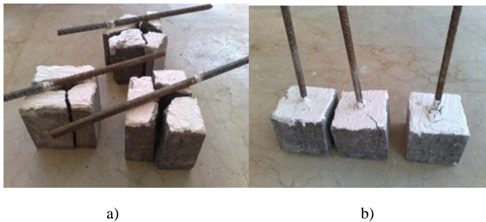
Figure 4.5 Typical failure patterns of concretes a) without steel fiber and b) with steel fiber
