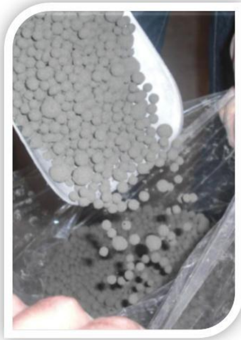
Figure A.5 Self-curing of fresh aggregate by kept it in sealed bags
