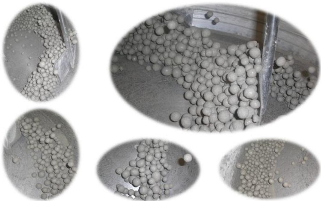
Figure A.4 Formation of fresh aggregate in pelletization process
