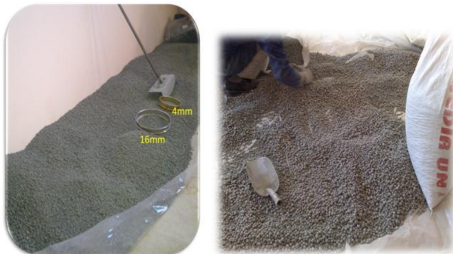
Figure 3.7 Hardened aggregate sieved by (16, and 4) mm sieve
