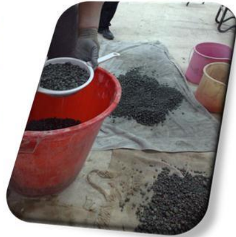
Figure A.7 Aggregate immersed in water for 30 min. to get SSD aggregate
