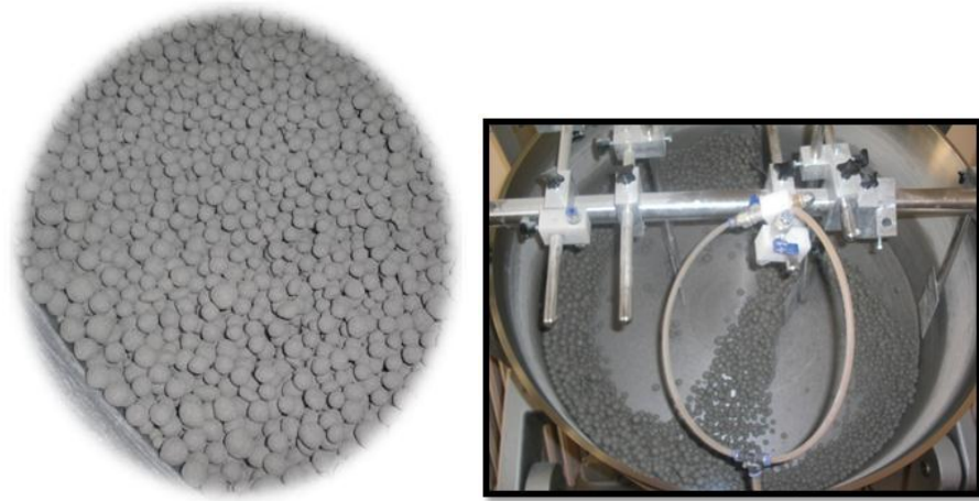
Figure 3.5 Spherical pellets formation after approximately 20 minutes
