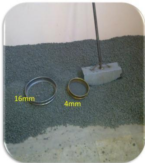
Figure A.6 Hardened aggregate sieved and ready for mixes
