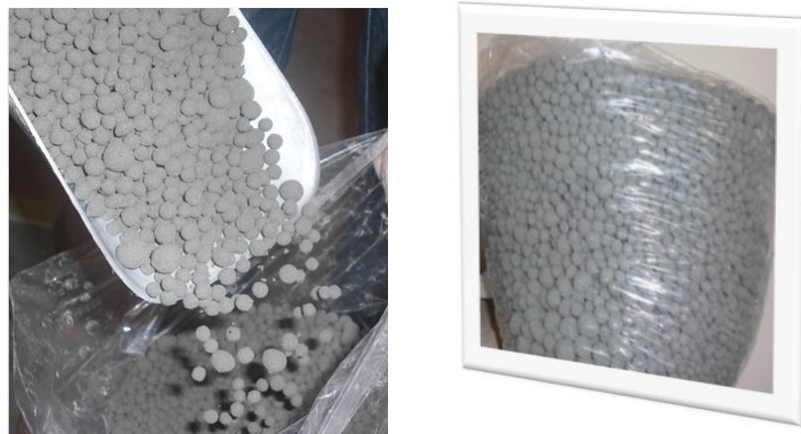
Figure 3.6 Air curing of fresh aggregates by keeping in sealed plastic bags
