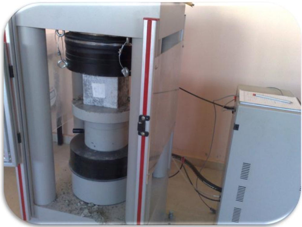
Figure A.9 Cubic specimen under compressive test
