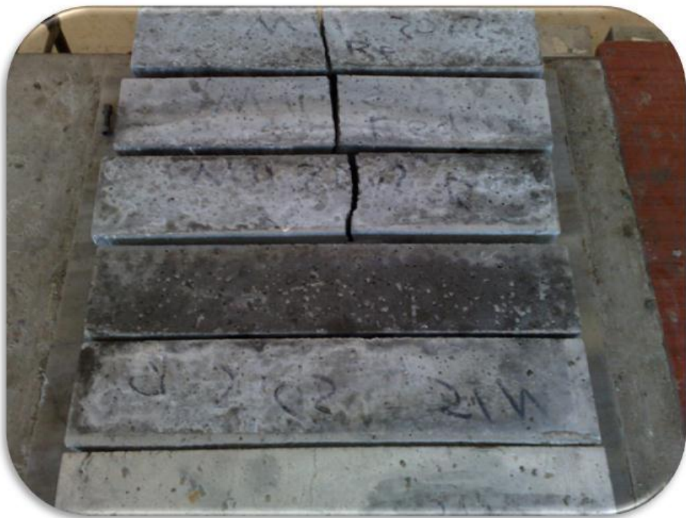
Figure A.10 Flexural specimens after testing for plain and steel fibers mixes
