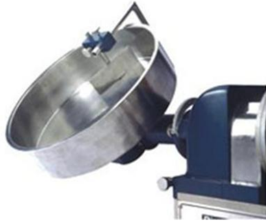
Figure 2.2 Disc pelletizer machine (Bijen, 1986)
