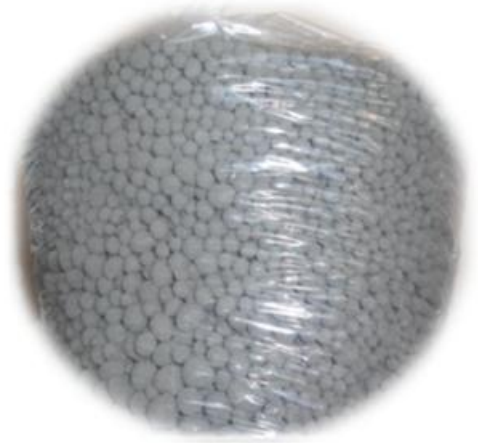
Figure A.5 Self-curing of fresh aggregate by kept it in sealed bags
