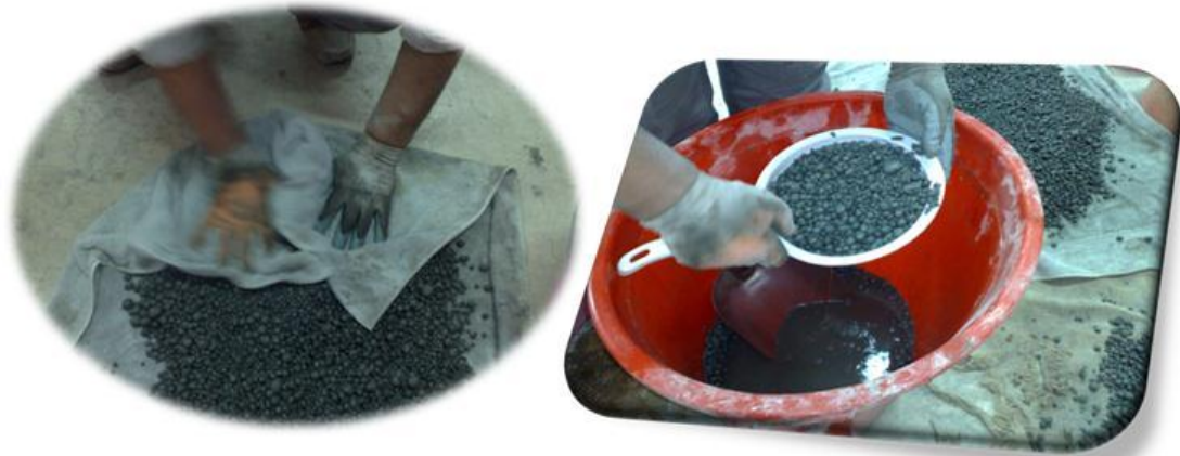
Figure A.5 Lightweight aggregate immersed in water before mix to get SSD aggregate (saturated surface dry aggregate)
