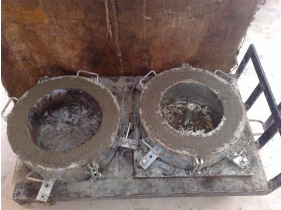
Figure A.7 Ring specimens after mixing, vibrating and finishing
