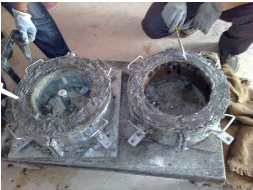
Figure A.8 Covering ring specimens by silicon rubber after 24h of casting
