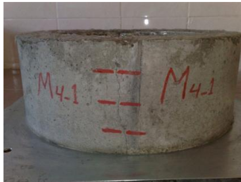
Figure 3.13 Photographic view of a cracked ring specimen (M4- 0.25% Steel fiber)
