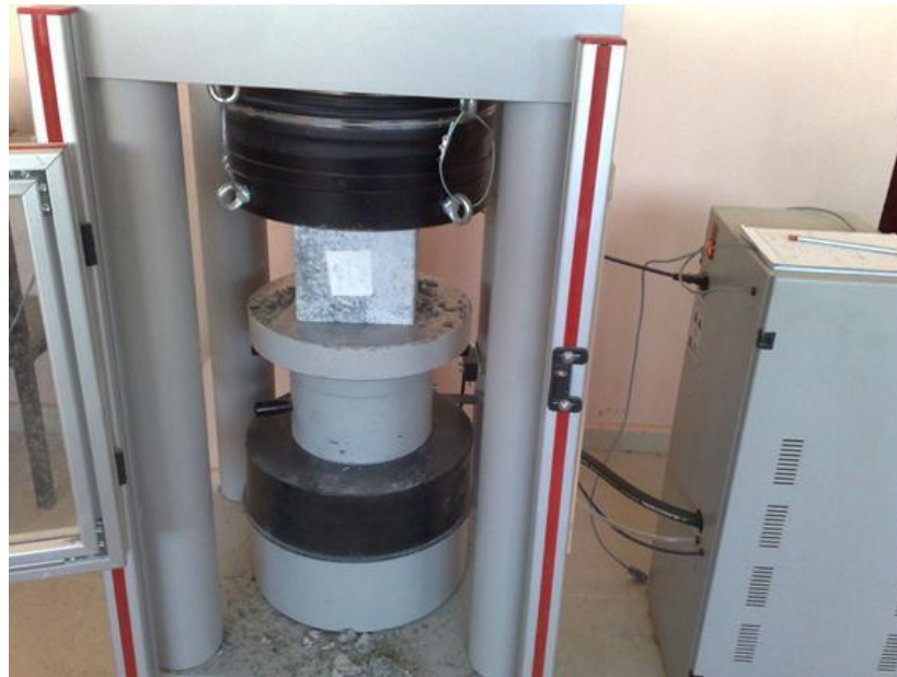
Figure 3.16 Photograph of compressive strength test
