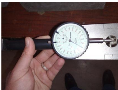
Figure 3.14 Dial gage extensometer for free shrinkage measurement (1 division = 0.002 mm)
